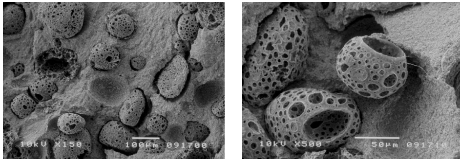
Figure 6.29 – Crosslinked composite with microcapsules mC-BH1 linked to the matrix through filaments of poly(HEMA).
