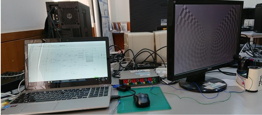
Appendix C Figure 1) System montage using one computer running both Matlab TM instances. The photodiode is placed on the lower right corner of the screen, coinciding with a frame identifying square imbued in each stimulation frame.
