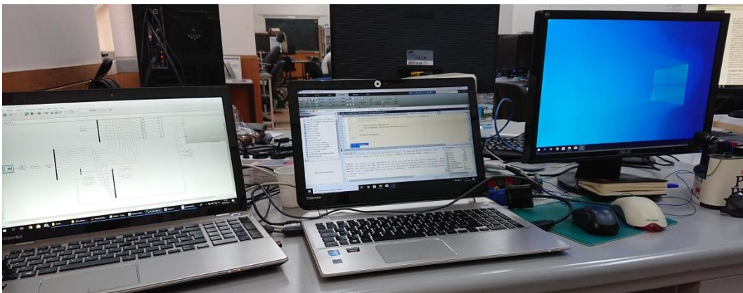
Appendix C Figure 2) System montage using two computers, each running one Matlab TM instance. The computers are connected through an Ethernet cable with an associated data transfer ping (in the millisecond scale).
