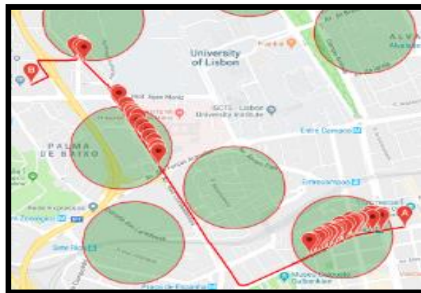
Figure 3.5 - Method of Maximum Overlap . At green, we have a base station in which call activity was detected. The figure is originally from Jundee et al. [35].
