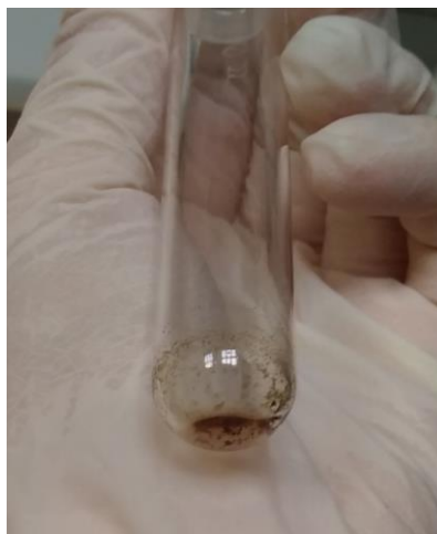
Figure 29. Undissolved suspended formed after dryness under nitrogen stream at 40 °C - Extraction F (Annex 10) and addition of MSTFA+5% TMCS.
