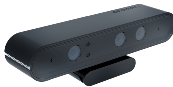
Figure 2.6: Orbecc Astra RGB-D sensor (reproduced from the Orbbec website).
