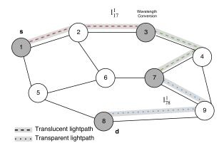
Fig. 1: The path from s to d is routed through the concatenation of  $l_{17}^1$  and  $l_{78}^1$ .
