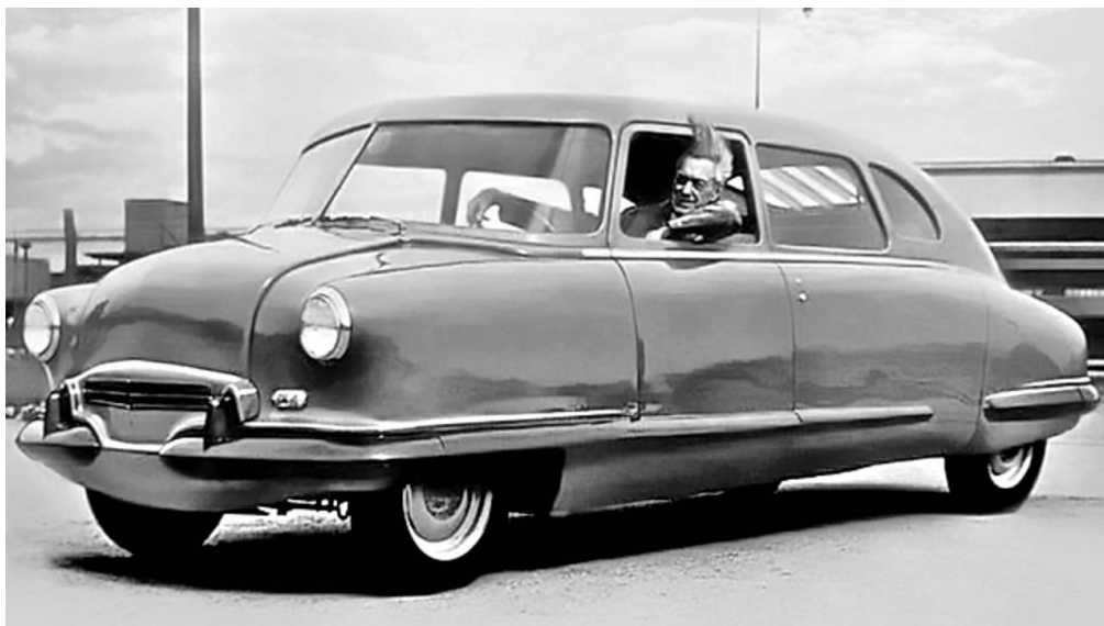
Figure 1.3 – Use of FRP composites in a car (Stout Scarab Experimental: first fiberglass-bodied car, 1946) [11]
