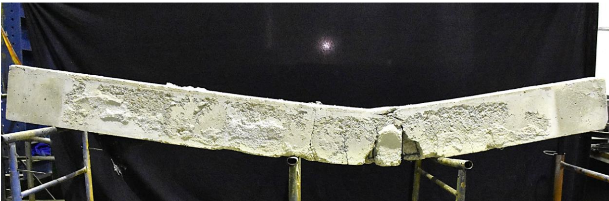
Figure B.5 – Failure mode of the OP-50 beam after fire resistance test
