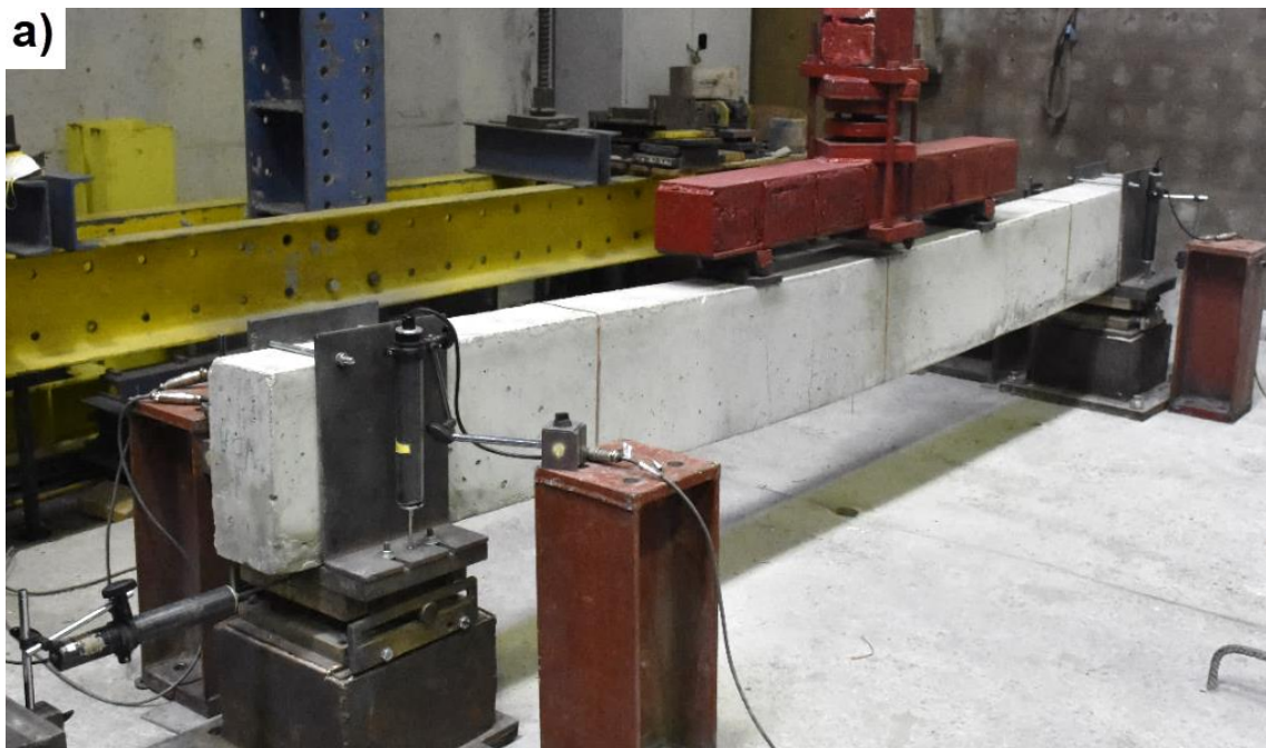
Figure 4.14 – Failure aspects of the CFRP-strengthened beam a few instants before strengthening collapse: (a) general view; (b, c) section with low displacements and initial cracking signals
