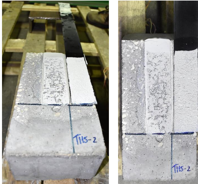
Figure A.7 – Failure mode in the adhesive at the CFRP-concrete interface for the T115-2 specimen tested at 115° C (perspective view on the left and front view on the right)
