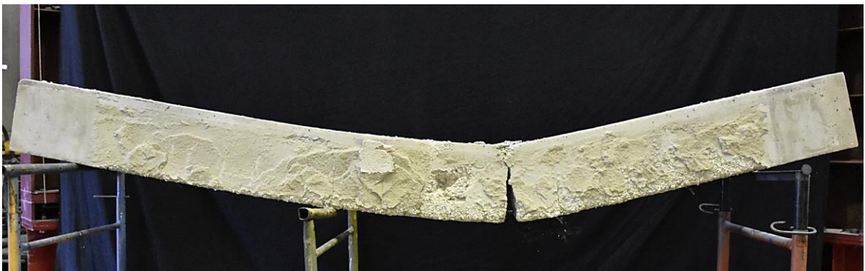
Figure B.2 – Failure mode of the EC-20 beam after fire resistance test
