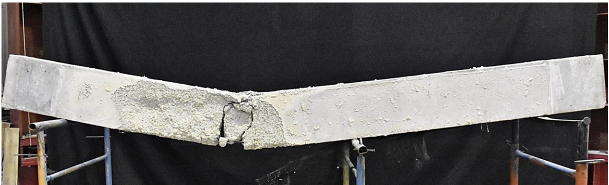
Figure B.7 – Failure mode of the VP-35 beam after fire resistance test
