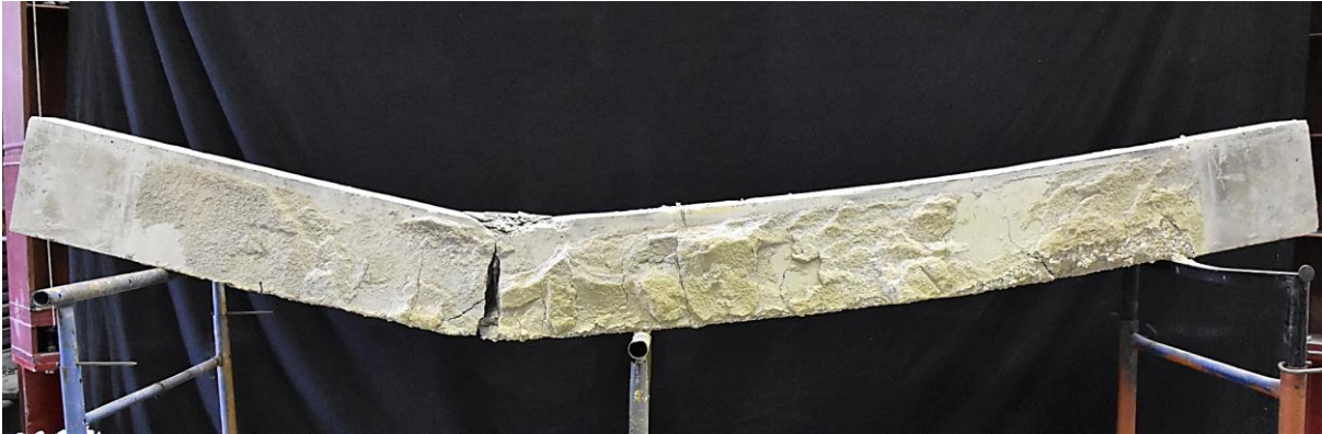
Figure B.3 – Failure mode of the EC-50 beam after fire resistance test
