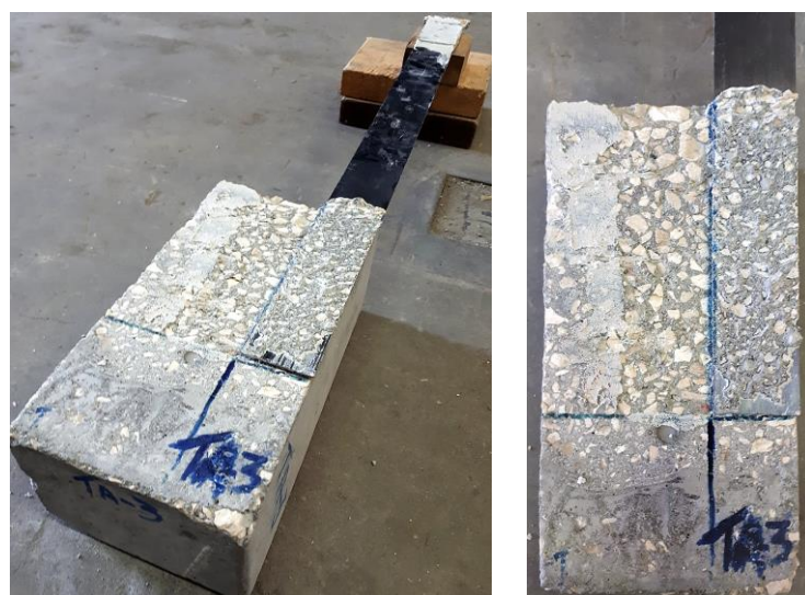
Figure A.2 – Failure mode in the concrete substrate for the TA-3 specimen tested at ambient temperature (perspective view on the left and front view on the right)
