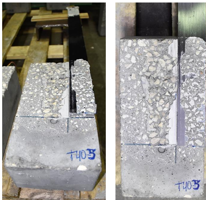
Figure A.4 – Failure mode in the concrete substrate for the T40-3 specimen tested at 40° C (perspective view on the left and front view on the right)
