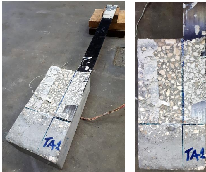
Figure A.1 – Failure mode in the concrete substrate for the TA-1 specimen tested at ambient temperature (perspective view on the left and front view on the right)
