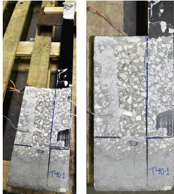
Figure A.3 – Failure mode in the concrete substrate for the T40-1 specimen tested at 40° C (perspective view on the left and front view on the right)
