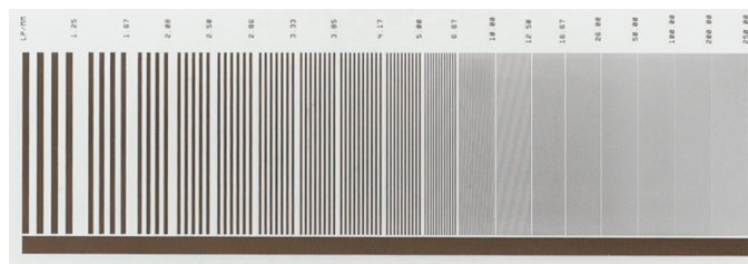
Figure 5.1 - Representation of variable line grating (Thorlabs).
