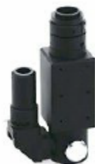
Figure 4.15 – Photograph of the infinity-corrected microscope module installed.
