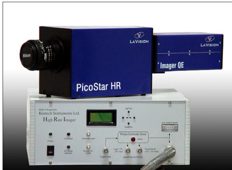
Figure 4.5 - The HRI (PicoStar HR) and HRI Controller Devices included in the LaVision image intensifier system. Our system uses a different CCD from the one attached in this picture (LaVision, 2007b).
