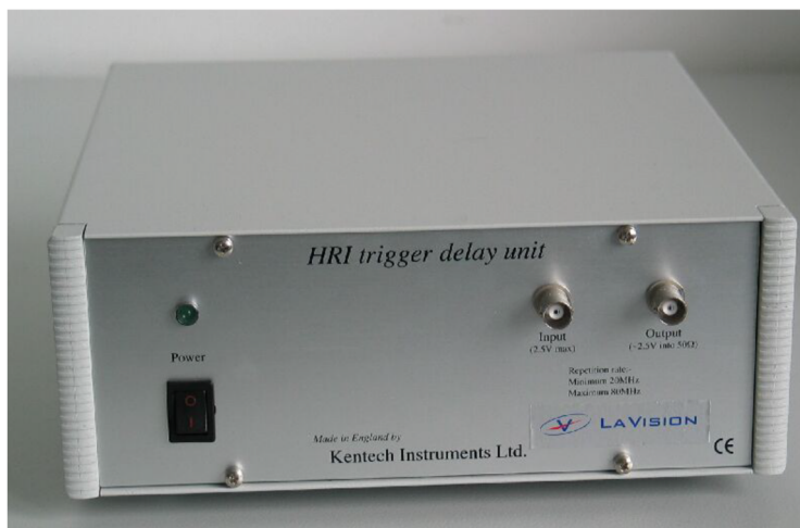
Figure 4.4 – The HRI Delay unit used in the Time-Gated acquisition system (LaVision, 2007b).
