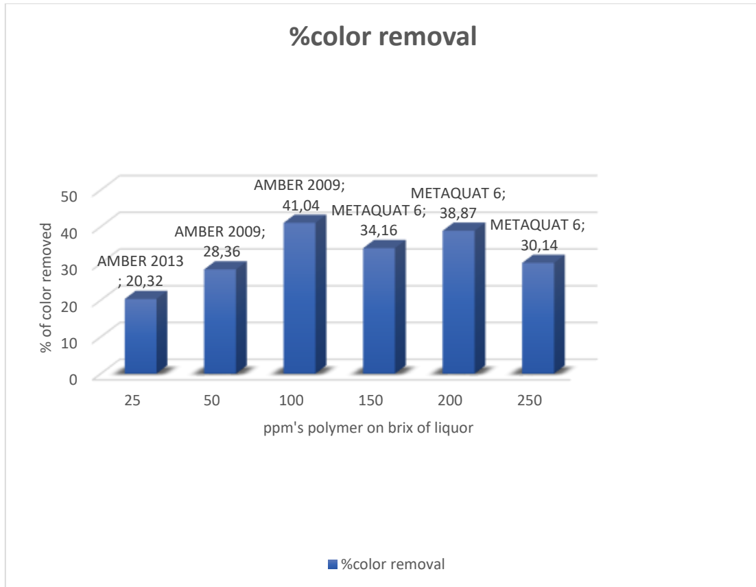
Figure 4.3: Graphic representation of the by the best performing polymer at each dosage and respective percentage of decolorization achieved.
