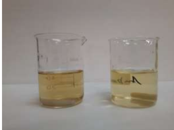
Figure 4.2: the filtrated liquor blank (on the left) and treated with the polymer Amber 2013 100ppm (on the right).
