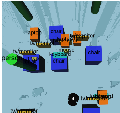
Figure 3.7: Semantic Map Visualization - At this point the system acknowledge the presence of 3 persons, 5 chairs, mouses, keyboards, monitors, etc.
