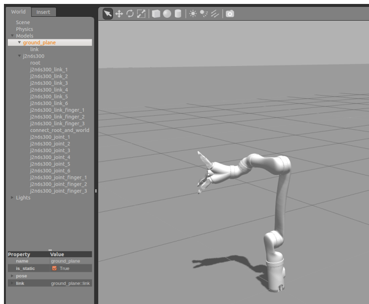
Figure 2.5: Kinova JACO 2 arm in Gazebo simulator.
