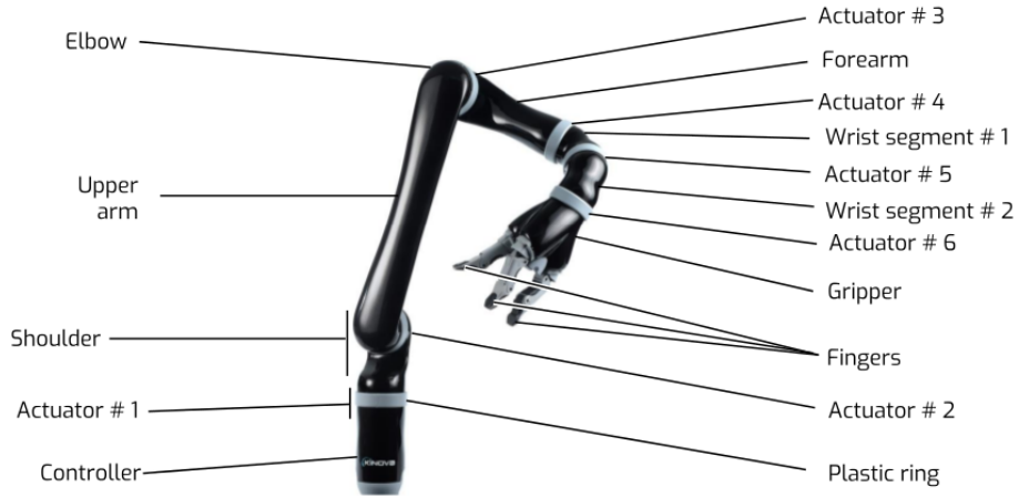
Figure 3.2: JACO 2 6DOF curved wrist components [7].
