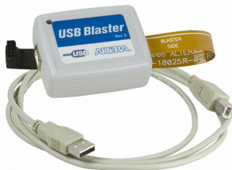
Fig. 3.4 Altera USB Blaster - Used to reconfigure the FPGAs through JTAG.
