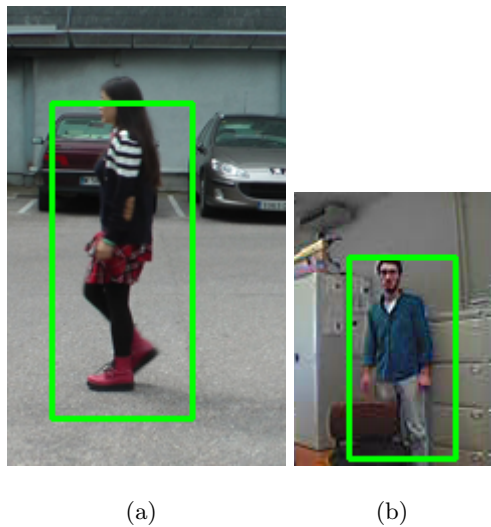
Figure 5.3: Result of the pedestrian detection on the sub-region of the original image (redefined ROI, with a pixel margin of 25 pixels for X80Pro image and 30 pixels for LASIESTA image).
