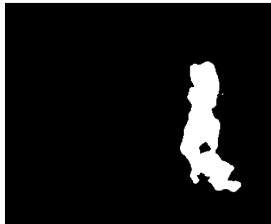
Figure 3.8: Binarized image following Otsu's threshold, applying Equation 3.8.
