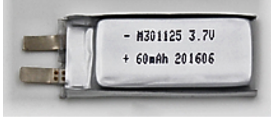
Figure A.3: Typical Lithium-Ion rechargeable battery. This one has a rated voltage of 3.7V.
