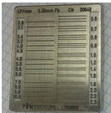
Figure 35: **MTF mask used as an imaging target:** this mask was made of 0.05 mm thick lead. Sets of three slits with variable separation (in lp/mm) allow the MTF estimation.
