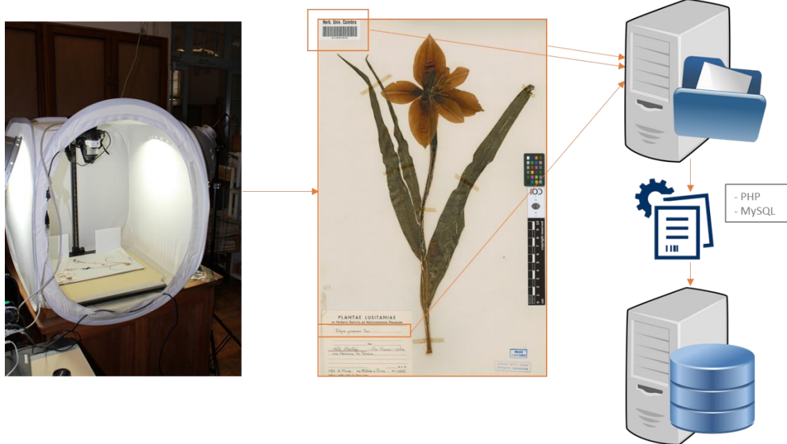
Fig. 18 - Automatic database procedures. After capture, the images are processed to create database records on SPECIFY. Copies and originals are stored in final directories.
