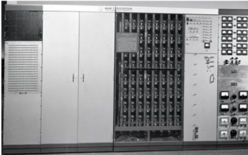
Figure 22 : Photograph of Mark I Perceptron machine of Rosenblatt, as seen at MIT exhibition.
