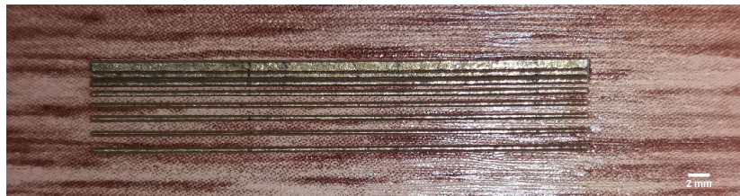
Figure 3.11: Stencil used for minimum feature separation test.
