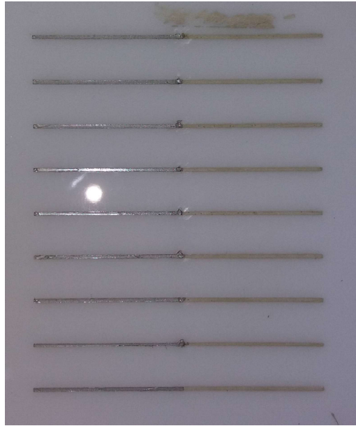
Figure 3.16: Experimental setup for characterisation of the vias, with eight 3cm long, 1mm wide lines per layer and two control lines (one in each layer) which are not connected.
