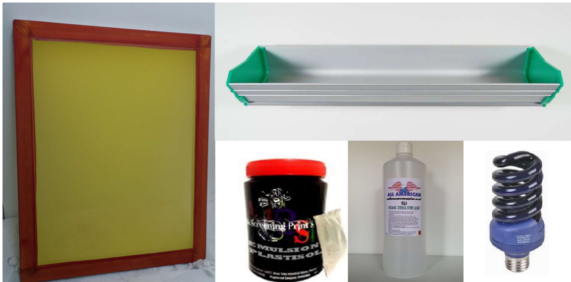
Figure 2.16: Screen (left); Coating through (top right); Photoemulsion (bottom center left); Emulsion remover (bottom center right); UV lamp (Bottom right).
