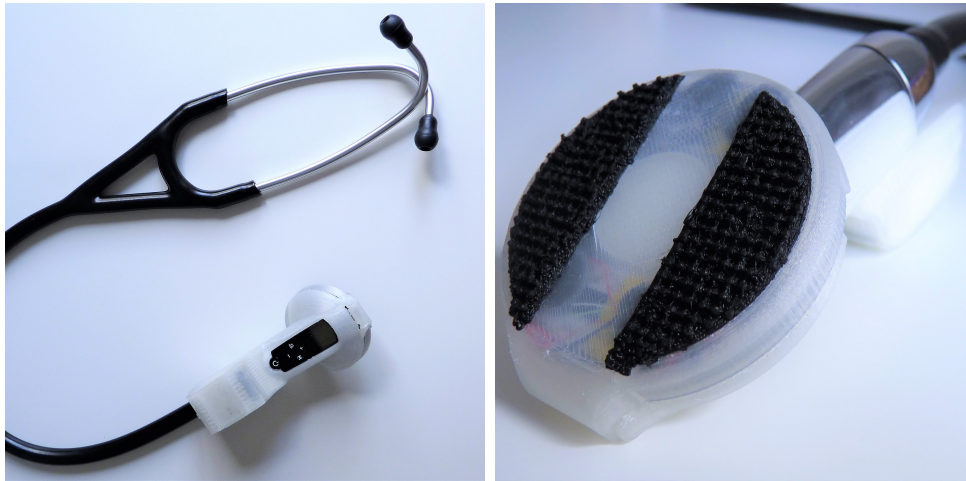
Figure 7.1: SmartHeart prototype model for ECG integration on a stethoscope.
