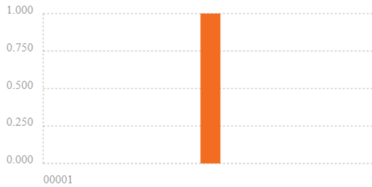
Figure 6.6: Output for the simulation of modular addition. The y-axis represents the probability of getting the bit register in the state shown in the x-axis.
