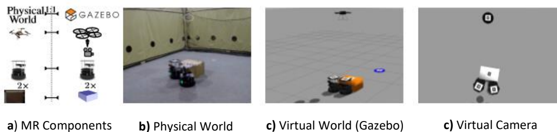
Figure 2.16 – Using Mixed Reality on simulation techniques. “Two TurtleBots collaboratively move a box using the guidance of a physical UAV with a virtual downward facing camera simulated with GAZEBO. The pose of the robots and the box are estimated using AR tag detection”. Image from (Hönig et al, 2015)
