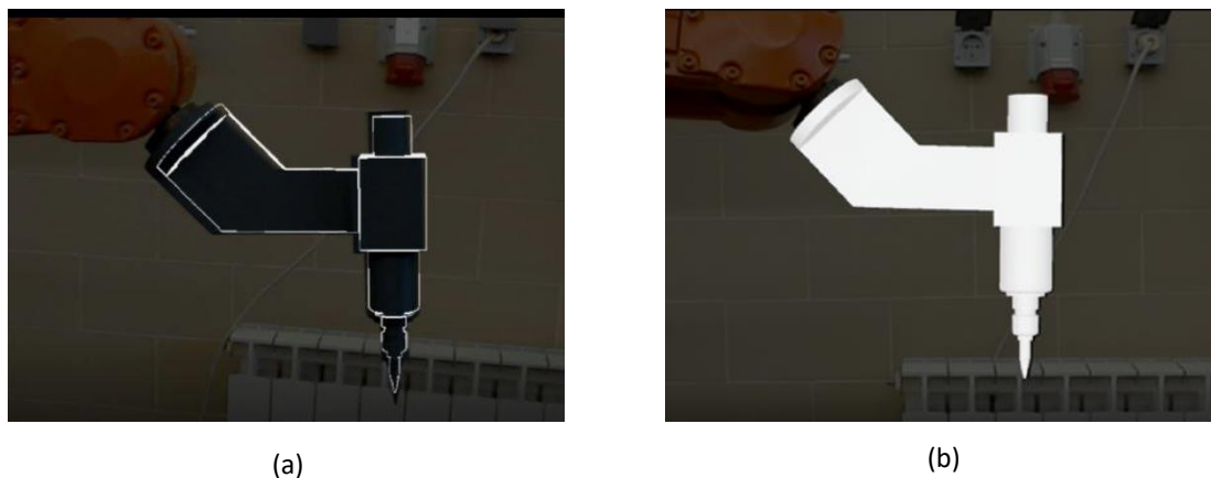
Figure 4.3 - Different stages of the Object tracking process in "Path Visualization" app: (a) Before tracking. Matching the guide lines with the real tool; (b) After tracking. Virtual object rendered on the real tool's position
