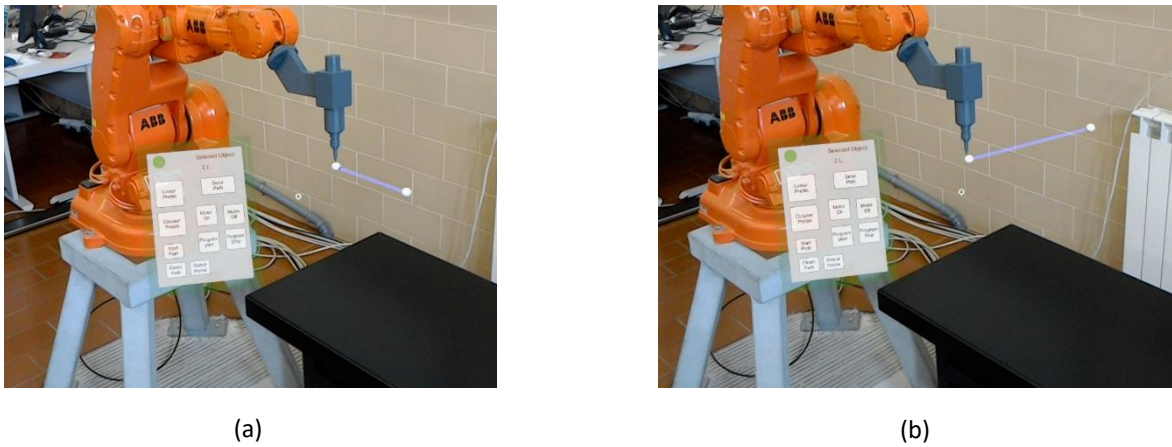
Figure 5.2 – Representation of linear movements as Holographic lines on the Graphical Path Manipulation app: (a) Holographic representation of a linear movement after its creation, without manipulation; (b) Holographic line after being manipulated by the user
