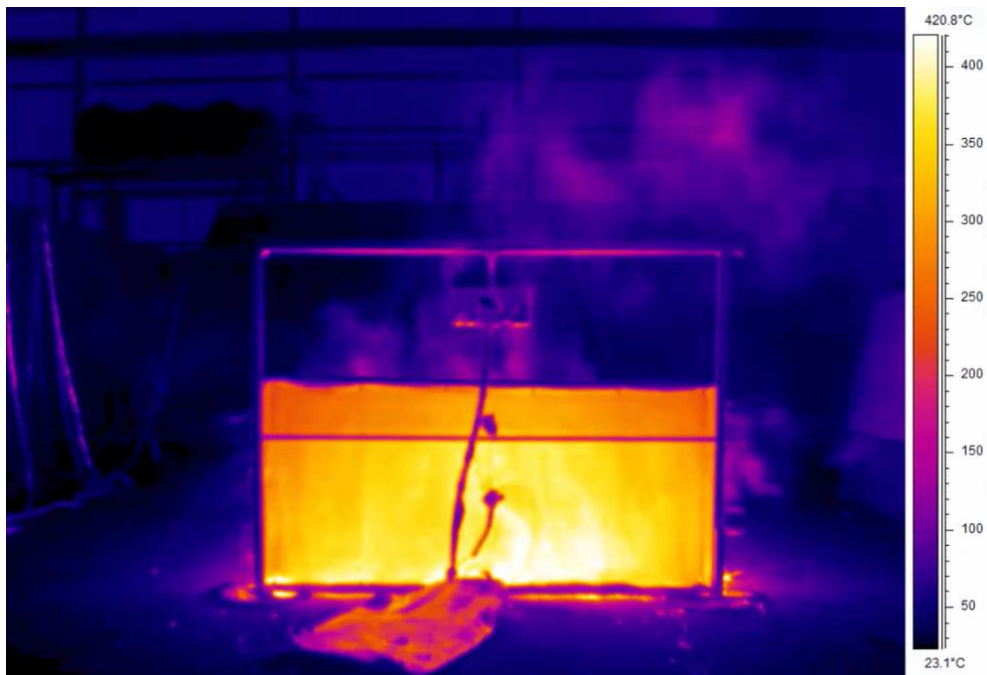
Figure 0.28. Maximum temperature recorded by the IR camera for wind speed ( U=2 m/s)
