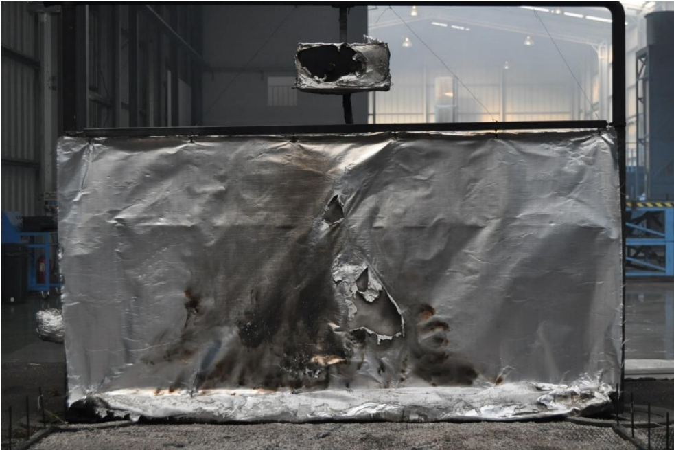
Figure 0.44. Tela2 at the end of the tests (wind speed, 1m/s; Fuel mass, 3.5 kg/m 2 )
