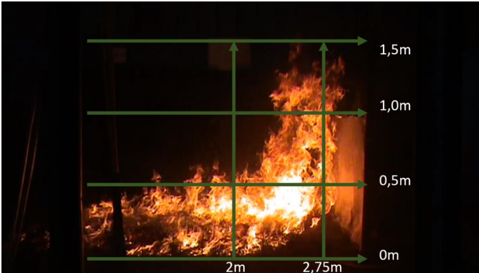
Figure 0.27. Flame height of Tela4 (U=1 m/s)
