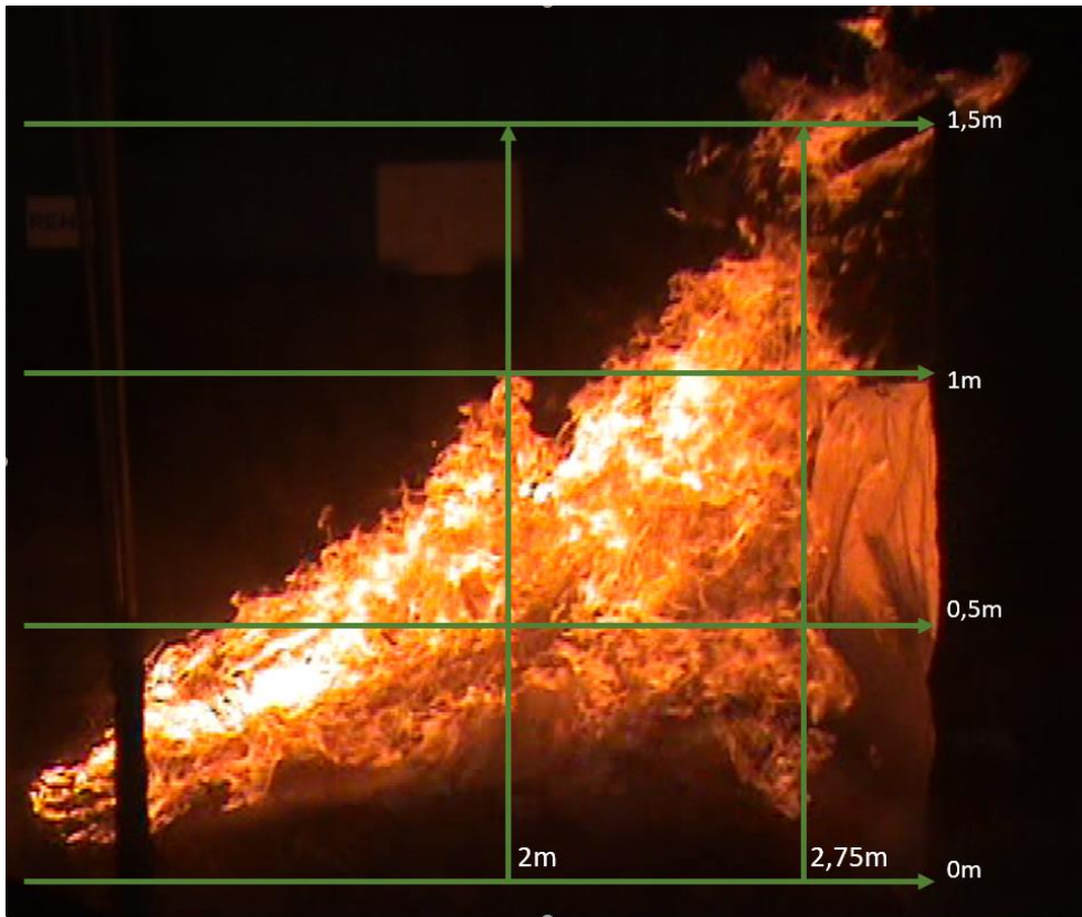
Figure 0.41. Flame height of Tela2 (wind speed, 3m/s; Fuel mass, 3.5 kg/m 2 )
