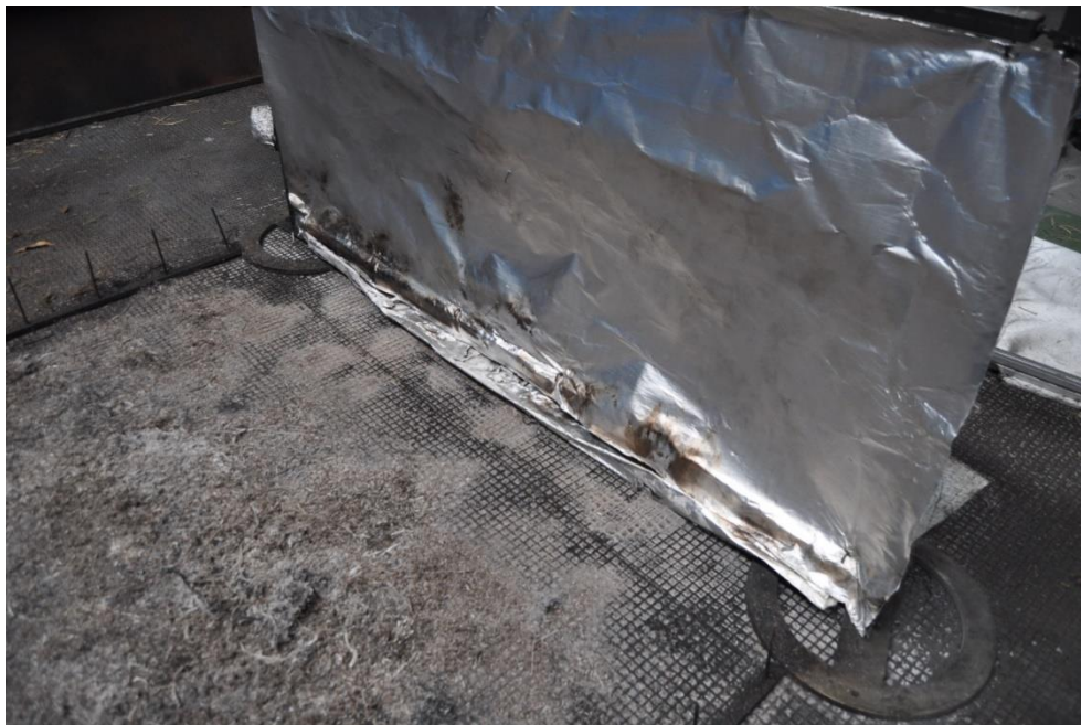
Figure 0.42. Tela2 at the end of the tests (wind speed, 3m/s; Fuel mass, 3.5 kg/m 2 )
