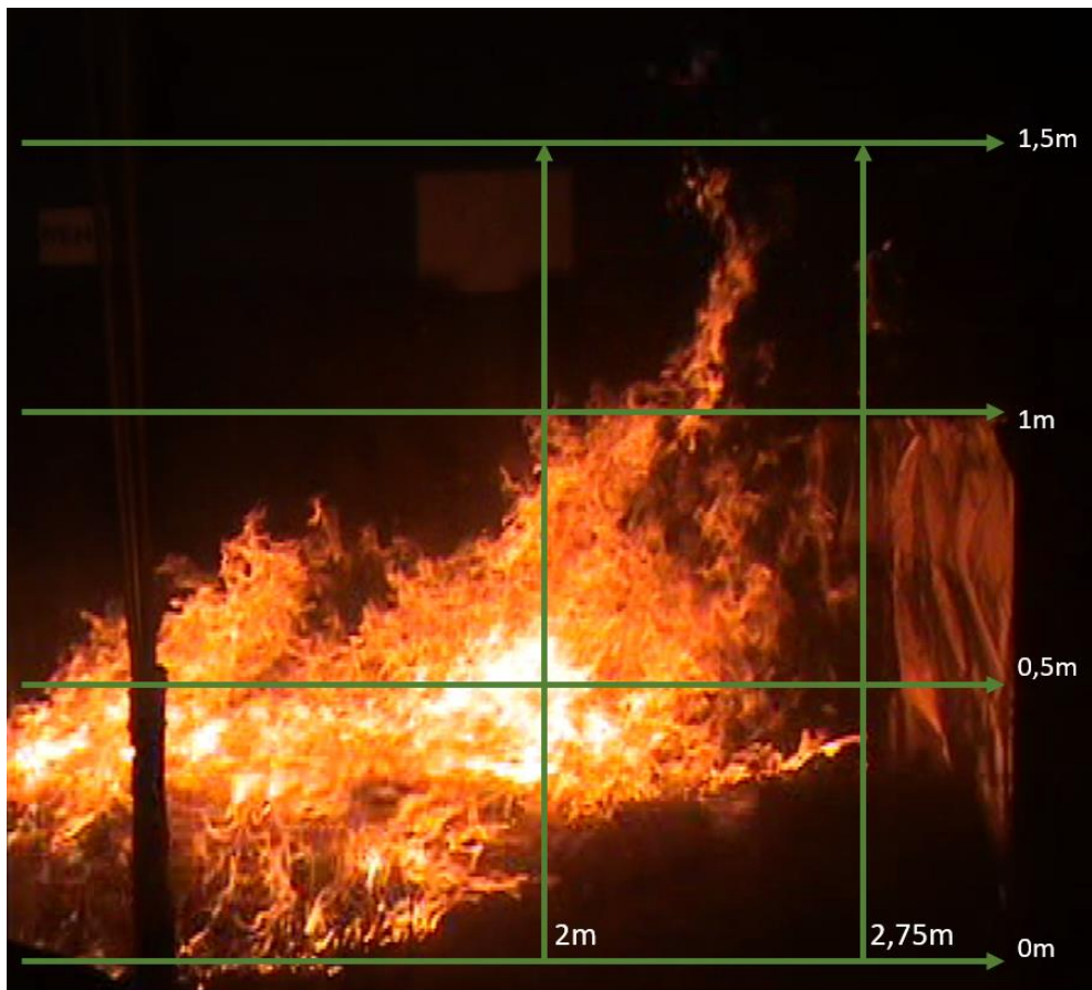
Figure 0.37. Flame height of Tela2 (wind speed, 3m/s; Fuel mass, 2.5 kg/m 2 )
