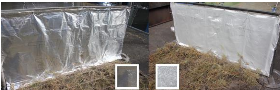
Figure 3.1. Fiberglass fabrics (with and without aluminium film)
