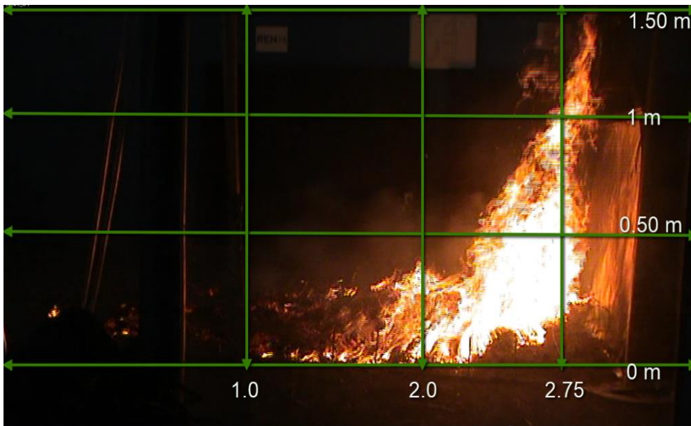
Figure 0.6. Flame height of Tela1 ( U=1 m/s)
