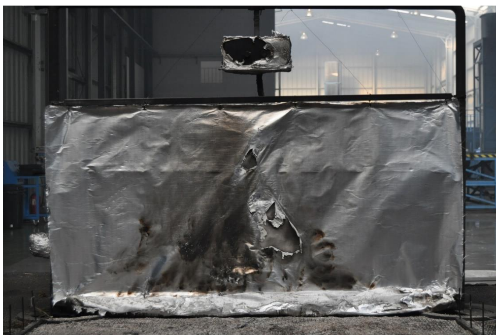
Figure 3.10. Tela2 at the end of the tests (wind speed, 1m/s; Fuel mass, 3.5 kg/m 2 )
