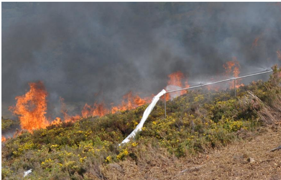
Figure 5.2. Fence and sprinklers (during first field test)
