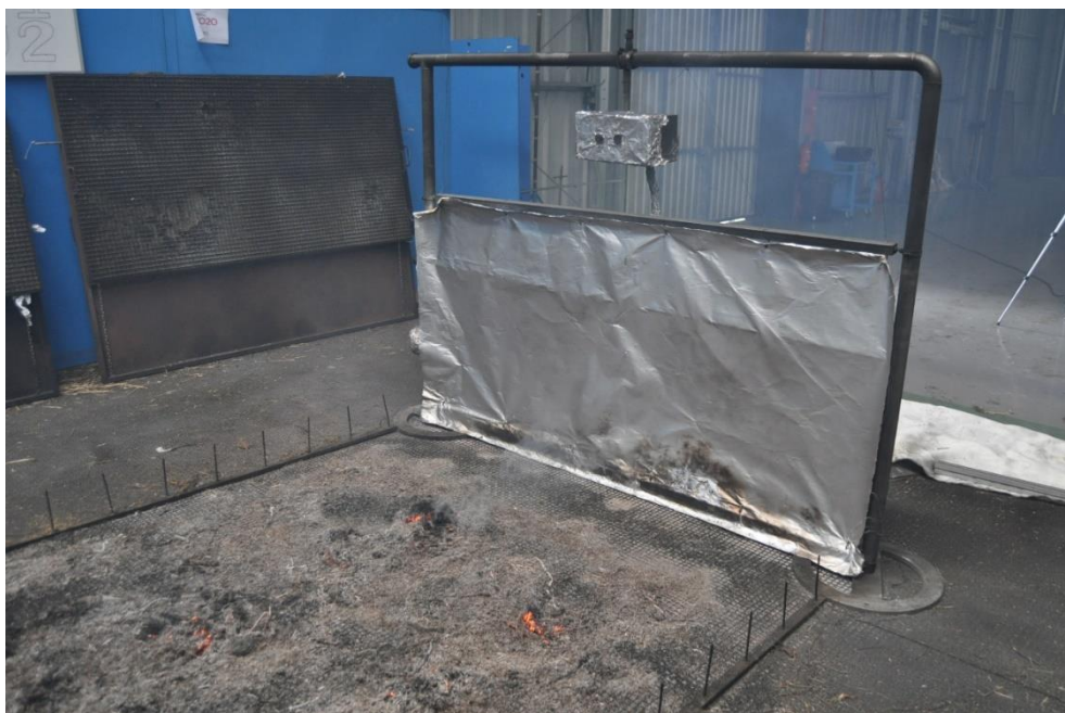
Figure 0.38. Tela2 at the end of the tests (wind speed, 3m/s; Fuel mass, 2.5 kg/m 2 )
