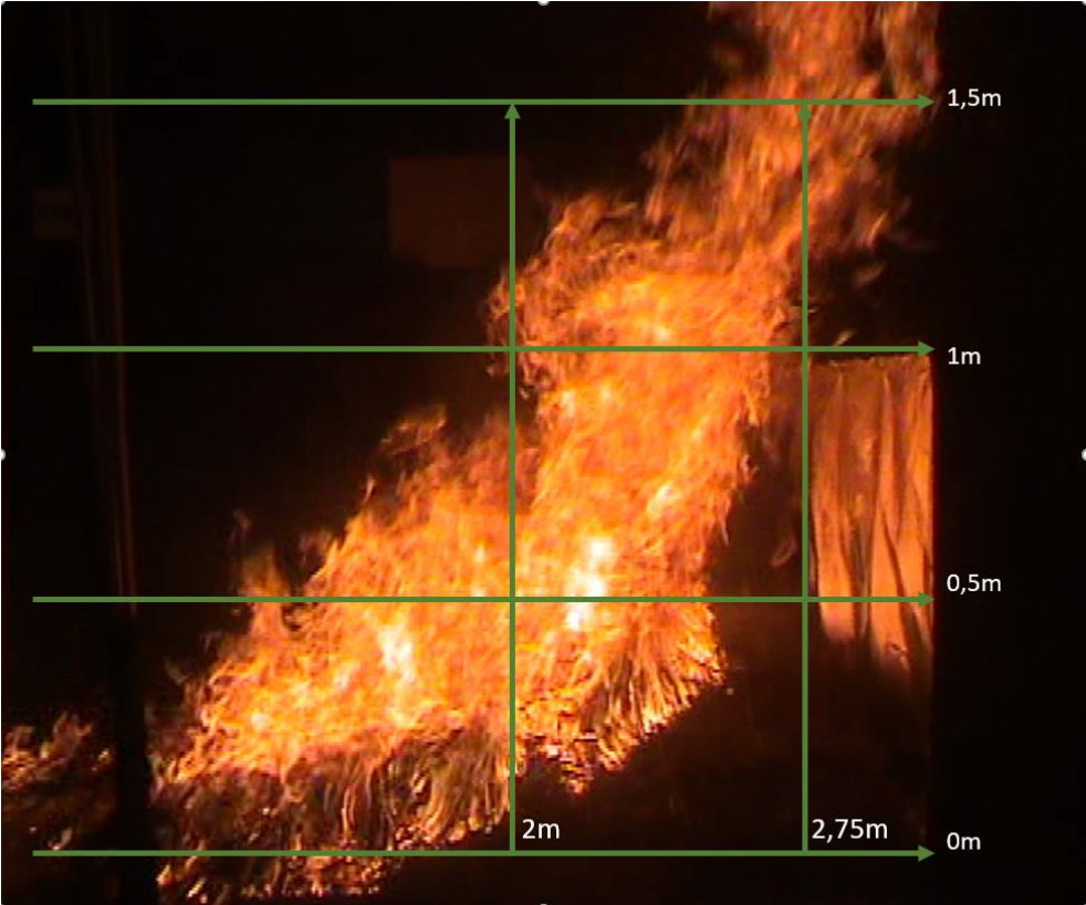
Figure 0.43. Flame height of Tela2 (wind speed, 1m/s; Fuel mass, 3.5 kg/m 2 )
