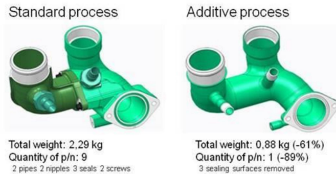
Figure 1.3 - Design for AM resulted in subpart elimination and weight reduction. (Ålgårdh et al., 2017)
