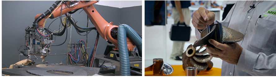
Figure 1.4 - a) Robot from MWES performing AM tasks. b) Propeller made with AM technologies. Source: (Anandan, 2017)
