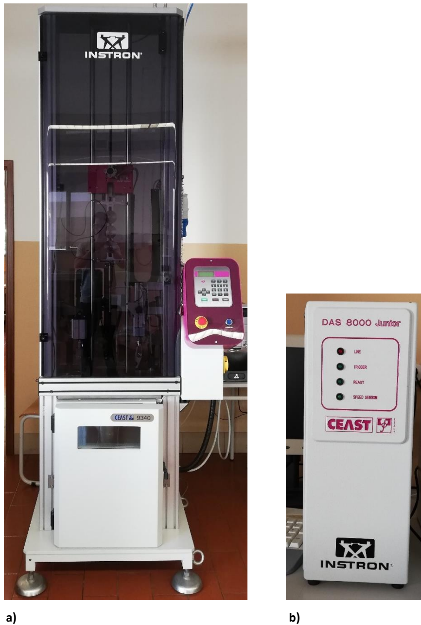
Figure 3.2. Equipment: a) Impact test machine CEAST 9340, and b) Data Acquisition System (DAS), both property of DEM (FCTUC).
