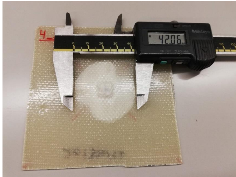
Figure 3.3. Calliper measuring visible damaged zone.
