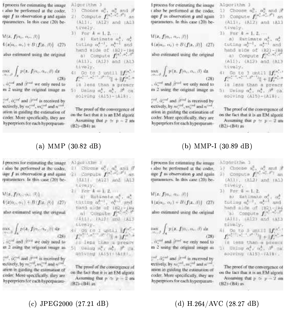
Figure 5.22: Detail for image PP1205 compressed at approximately 0.65 bpp using a) JPEG2000 and b) H.264/AVC.
