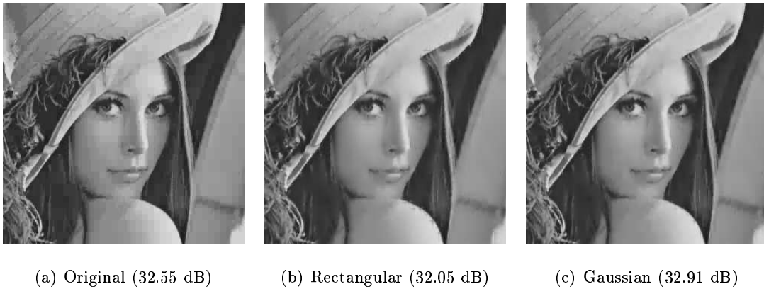
Figure 4.6: Detail of the MMP post-processing deblocking filters for image Lena coded at 0.29 bpp: a) MMP decoded image b) deblocking with rectangular kernel and c) deblocking with a Gaussian kernel.
