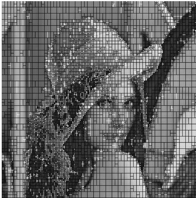
Figure 5.16: MMP-I segmentation for image Lena coded at 0.5 bpp. The prediction blocks are represented by the black lines and the MMP segmentation is represented by the white lines.
