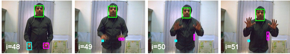
Figure 3.9: Effect of fast motion while tracking three skin-colored objects. Frame 48) Both hands are in rest position and tracked (cyan = right hand; pink = left hand). Frame 49-51) Hands are lifted with a fast motion and the tracker gets 'stuck'.
