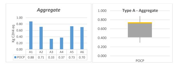
Figure 6.5 – Benchmarking of aggregate results of the life cycle environmental assessment normalised per m<sup>2</sup> of the deck
