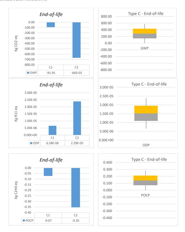
Figure 6.16 – Benchmarking of end-of-life stage normalised per m<sup>2</sup> of the deck
