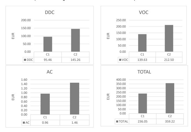
Figure 5.18 – Results of LCS of bridges of Type C normalised per  $\mbox{m}^2$  of the deck
