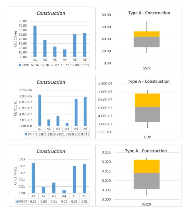
Figure 6.2 - Benchmarking of construction stage normalised per m<sup>2</sup> of the deck
