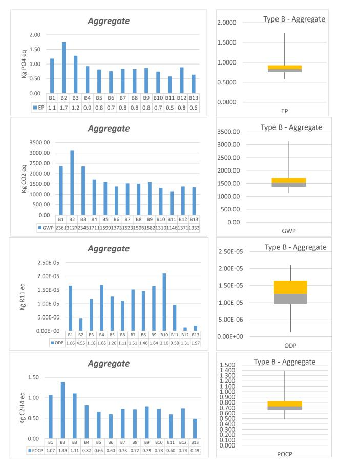
Figure 6.11 – Benchmarking of the aggregate results normalised per m² of the deck
