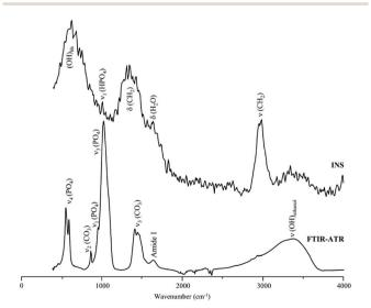
Fig. 4 FTIR-ATR and INS spectra of enzyme-treated human femur. The INS data was measured in the MAPS spectrometer (with a 5240 cm<sup>-1</sup> incident energy).
