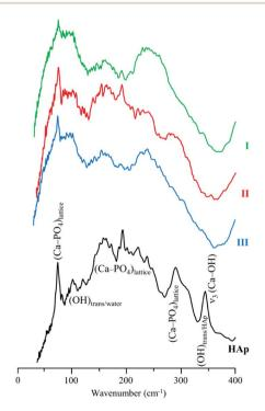
Fig. 5 Low energy INS spectra of human femur, measured with the TOSCA spectrometer: intact (I), hydrazine-treated (II) and enzymetreated (III). The spectrum of reference calcium hydroxyapatite (HAp, SMR2910b) is also shown, for comparison,
