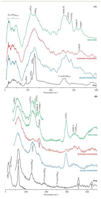
Fig. 3 INS spectra of human femur – intact, hydrazine- and enzymetreated – measured in two different spectrometers: (A) TOSCA and (B) MAPS (with 2024 and 5240 cm<sup>-1</sup> incident energies).
