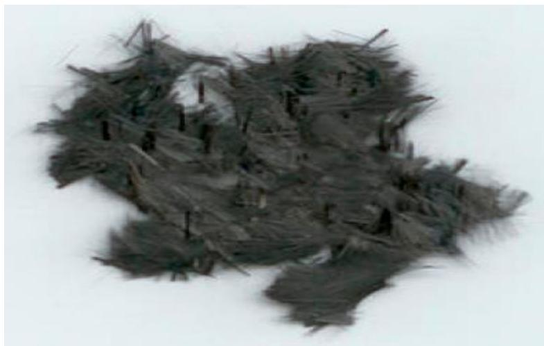
**Figura 2.12.** Fibra curta de carbono “*short carbon fiber*” [Apply, Procotex, 2015] .
