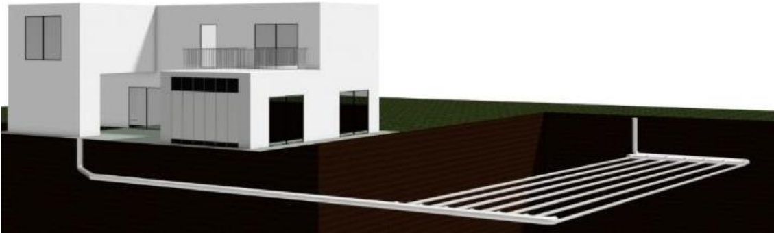
Figure I.2 – Earth-to-air heat exchanger and Water Trombe Wall in a LSF building.
