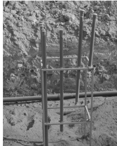
b) PVC pipes to insert the ground temperature probes at different depths.
