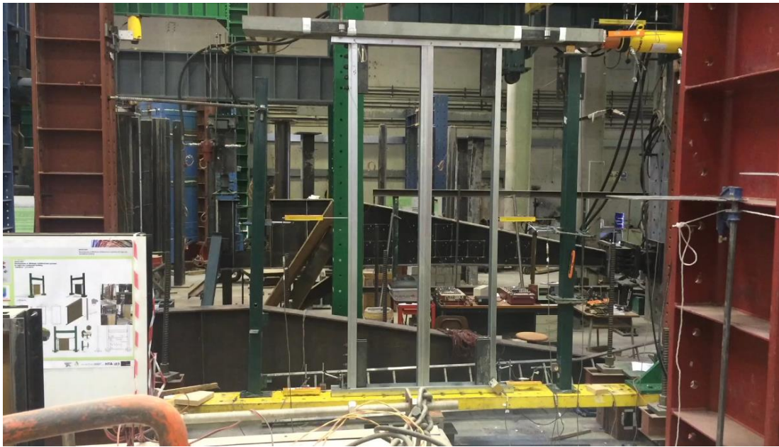
Figure I.1 – Experimental test with non-braced wall panels.
