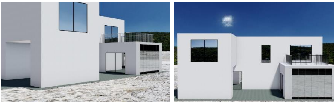
Figure VIII.27 – Tri-dimensional rendering of the water Trombe wall with six modules in a LSF construction (Cool Haven).
