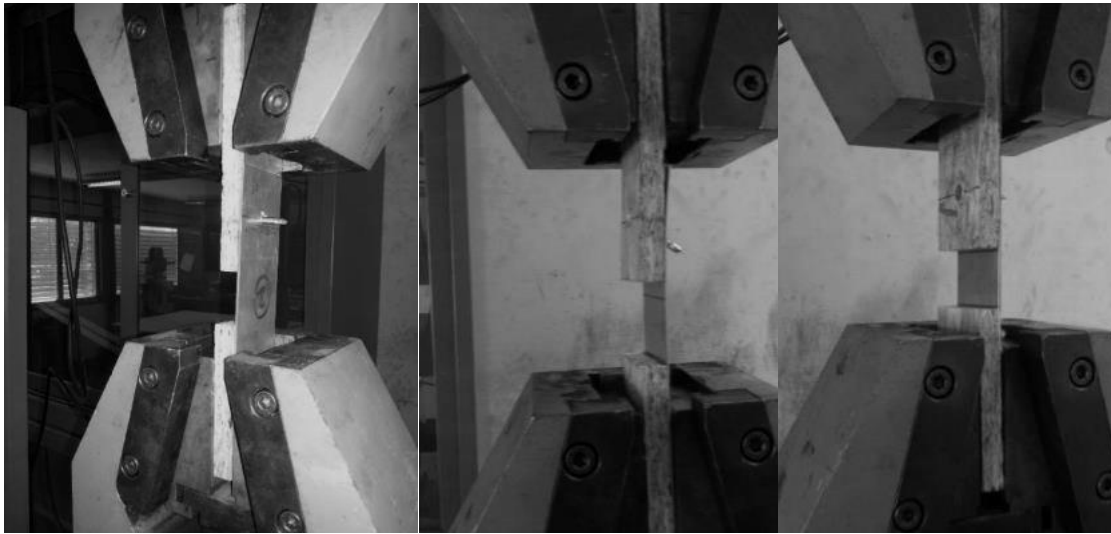
Figure III.21 – Experimental results for steel-OSB connection with ST 4.8 x32 screw.
