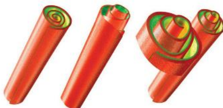
Figure 1 3D representation of rolled halloysite nanotubes, which are composed by two layers: alumina in the inner layer (green) and silica in the outer surface (red). Source: Lvov et al 6
