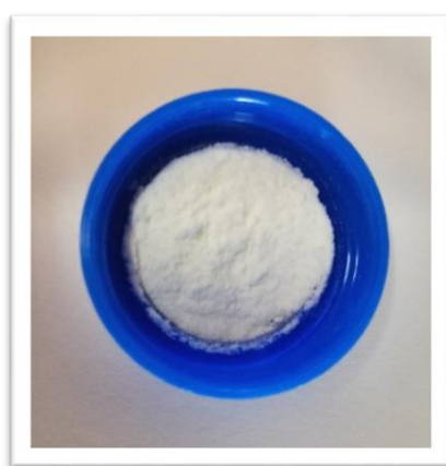
Figure 27: Atomized hybrid NLC powder obtained by spray-drying.
