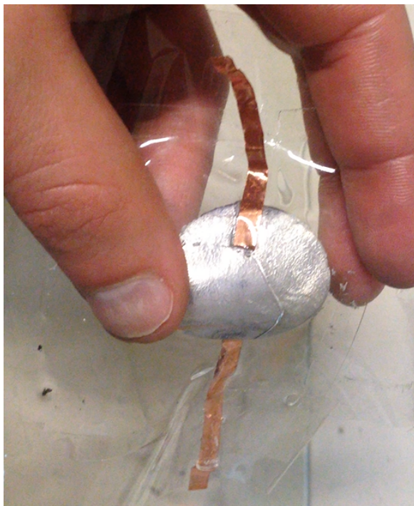
(a) Electrode fracture on top side
