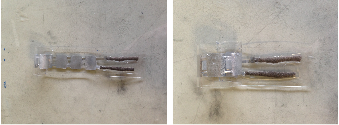
(a) Equilibrium position with the DEA adhered to the surface (b) Equilibrium position with the DEA curled
