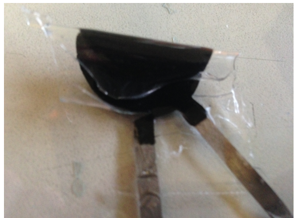
(f) Fissure near the connection upon stretching
