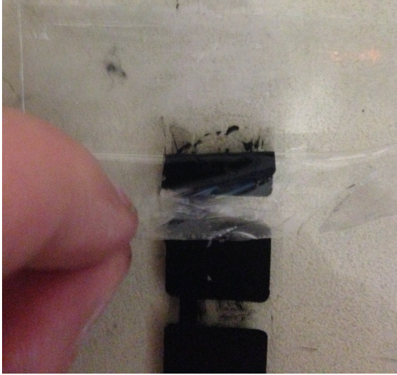
(a) The membrane is too glued to the surface on the electrodes places
