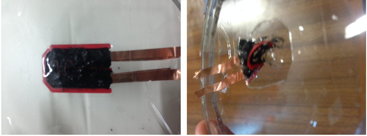
(a) Fingertip carbon grease electrodes with a VHB backing foil as a frame.
