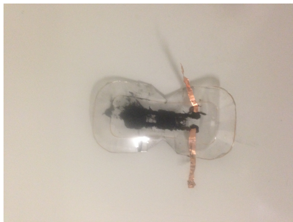
(c) Cuts are done to require less force to move the actuator
