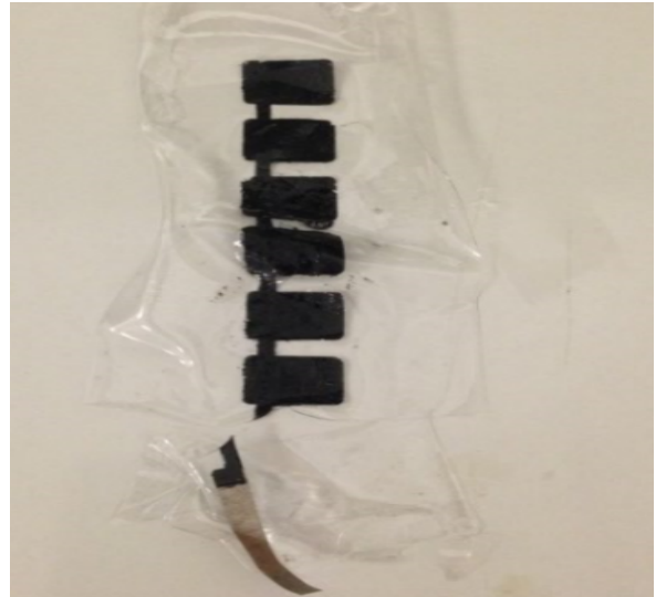
(d) Electrodes are encapsulated by PDMS; rupture near the connection
