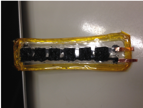
(c) Frame shrunk after going to the oven; carbon grease does not cure and it blurs easily
