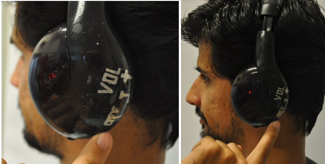
Fig. 4.10 Capacitive headphone. User pressing "On" bottom to turn the device on, turning the red LED active.
