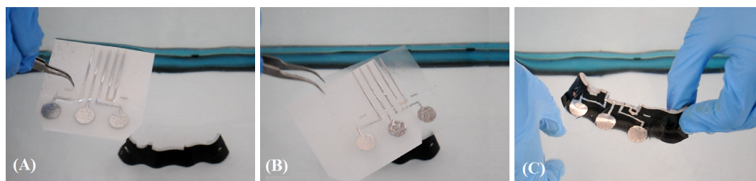
Fig. 4.5 (A) TTP with printed circuit and LED floating in the water. The host piece is submerged, (B) Protective back layer from TTP detaching, (C) Attaching the TTP film to the host piece.
