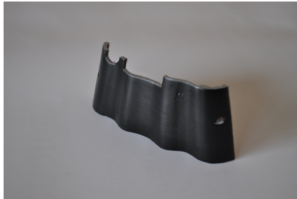
Fig. 4.1 3D printed piece to fit in a robotic prosthetic hand.
