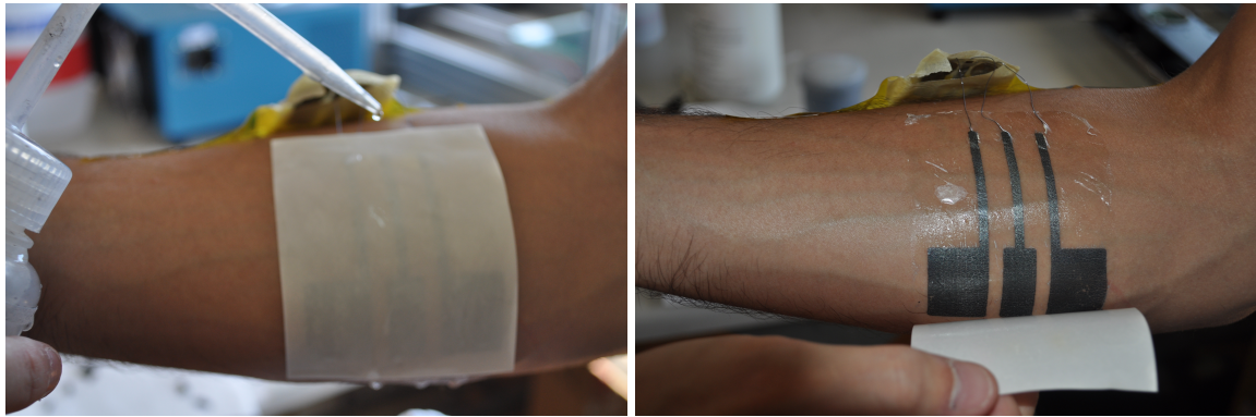
Fig. 4.14 (A) Watering the protective back layer of the TTP, (B) Peeling off the protective back layer, leaving the electrode exposed due to the film transparency.
