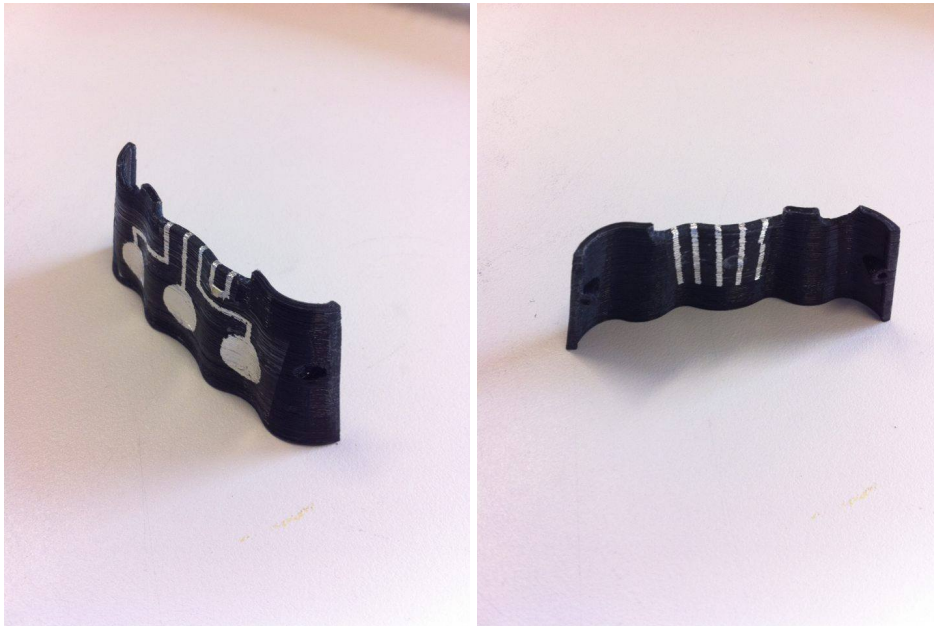
Fig. 4.6 Final result after transferring the TTP film to the host piece, showing the front and back respectively.
