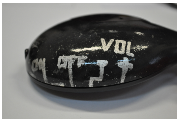
Fig. 4.11 Capacitive headphone bottoms with conductive traces bending to the inside part of the headphone case.
