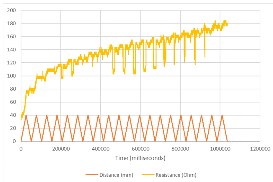
Fig. 3.25 Result of one sample test. Orange trace represents the average resistance and the red trace the distance travelled ( 40\text{mm} ) from the original position on each repetition cycle.
