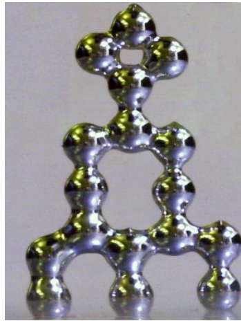
Fig. 3.7 Liquid Metal deposition due to oxide layer.
