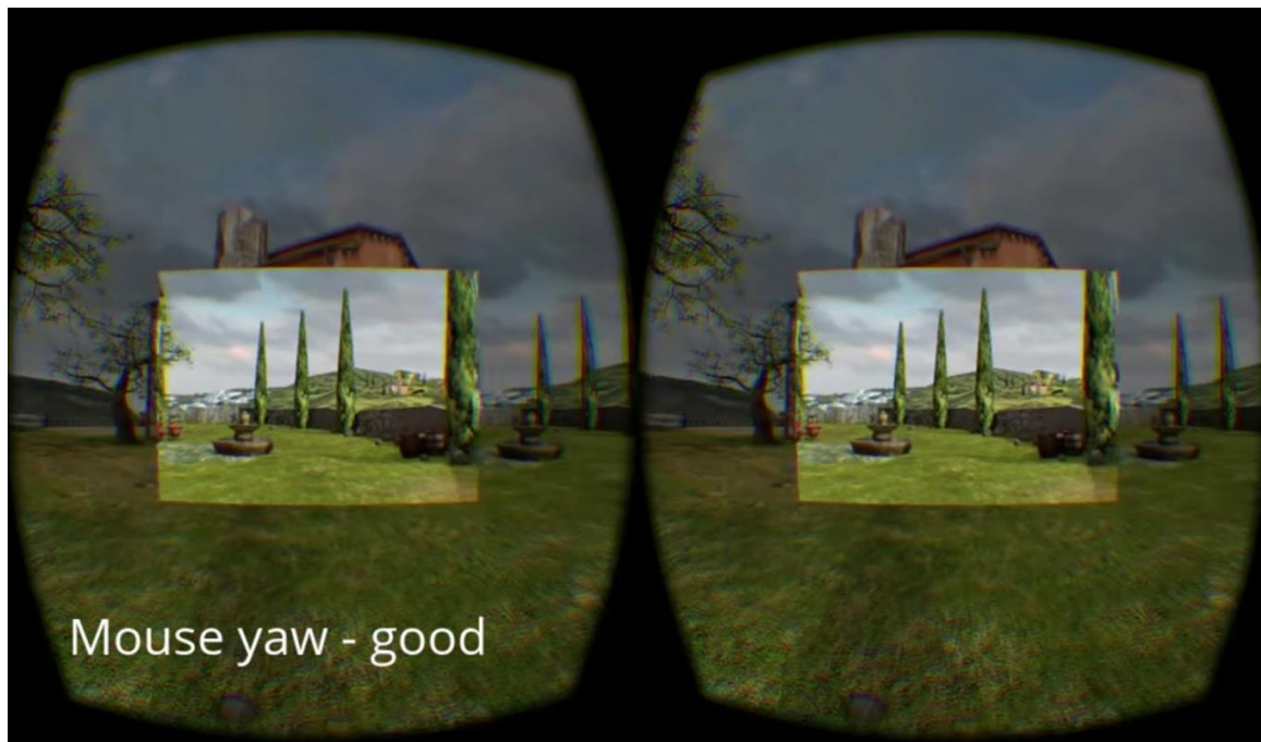
Figure 14 - Representation of Tunneling
