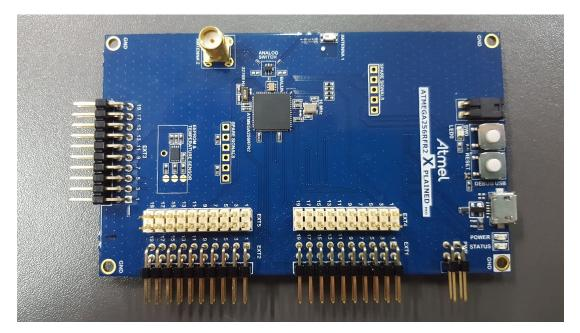
FIGURE 4.2: Atmega256rfr2 X-pro board
