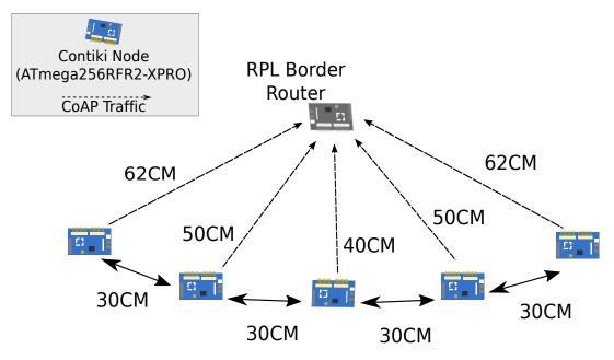
FIGURE 4.4: Clock drift evaluation scenario
