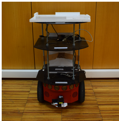
Figure 5.1: Robot Pioneer P3-DX, which is the type of robots used throughout this work.
