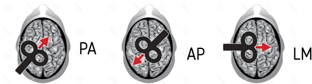
Figure 1.5 -TMS coil orientation can give rise to 3 induced-currents orientations. PA induced-currents are produced when the handle of the coil points backward at ~45° from the midsagittal line, and AP induced-currents are elicited by placing the coil 180° from the PA direction. LM induced-current direction is achieved by pointing the coil handle laterally. Adapted from [43].
