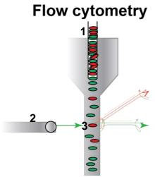
Figure 17. Flow cytometer analyser principal components. 1) nozzle; 2) laser beams; 3) cell containing a fluorescent tag that is excitable by the laser
