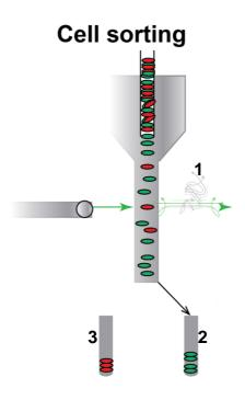
Figure 19. Cell sorter components mediating cell separation. 1) electric charge; 2) cells of interest; 3) remaining cells
