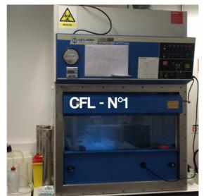
Figure 10. Vertical laminar flow chamber from Gelaire
