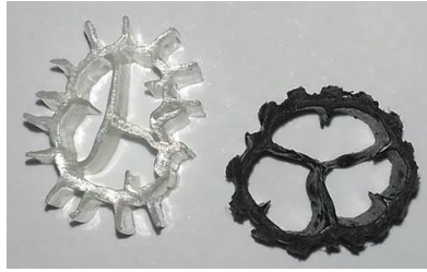
Fig. 5.2: Carrier comparison; new (left) vs one with about 10 years of utilization (right)
