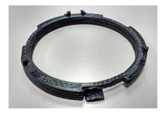
Figure 2.10: Spacer used to place the camera under the lens cup
