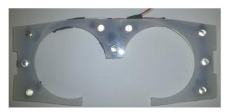
Figure 2.6: Acrylic plate with IR LEDs
