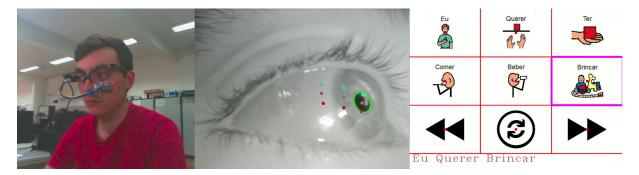
Figure 3.15: From left to right: User wearing the eye-tracking glasses, view of the users eye and virtual keyboard seen by the user
