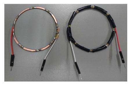
Figure B.4: Finished illumination rings. Left: bare copper, right: insulated with tape
