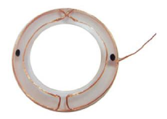
Figure 1.6: Contact lens with embedded coil used for eye tracking [18]
