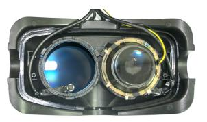
Figure 2.16: Detail of the HMD with one lens removed to show the camera
