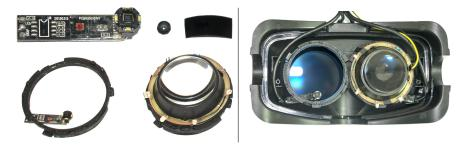
**Fig. 1.** Left: Camera board and sensor with 90 degrees bent connections; Lens; IR filter (film); Lens on spacer with IR ring; Spacer with camera below; Right: Oculus Rift DK2 with left lens out, showing spacer and camera installed; on the right we can see the illumination ring in mounted on the respective lens.
