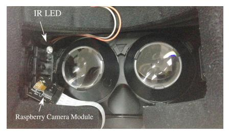
Figure 2.3: Eye tracking hardware setup using the Raspberry Pi
