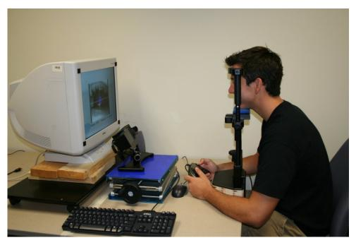
Figure 1.7: VOG type Eye tracker with head rest [19]
