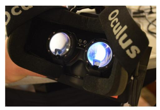
Figure 1.9: Oculus Rift upgraded with the SMI eye tracking package [26]
