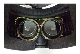
Figure 2.15: HMD with both cameras mounted and with the IR ring
