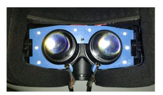
Figure 2.8: New plate with both illumination and camera brackets
