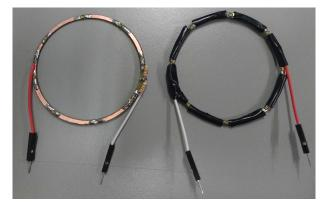
Figure 2.14: Illumination rings. Left: bare copper, right: insulated with tape
