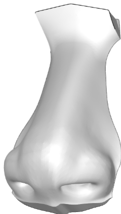
Figure 1.3: An example of an object to be produced with SLM technology. This is a nose and due to its geometry it is expected to be difficult to produce such object.
