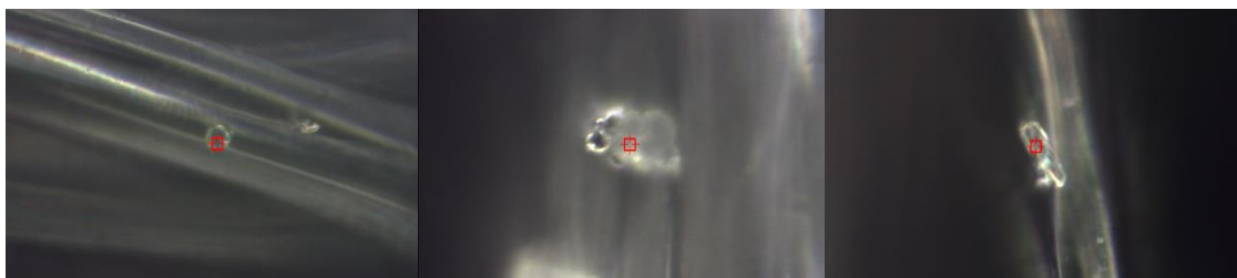
Figure 35. Left to right: particle of potassium chlorate (100x), ammonal (ALAN) (100x), and HMTD (100x) trapped in the white polyester fibres.
