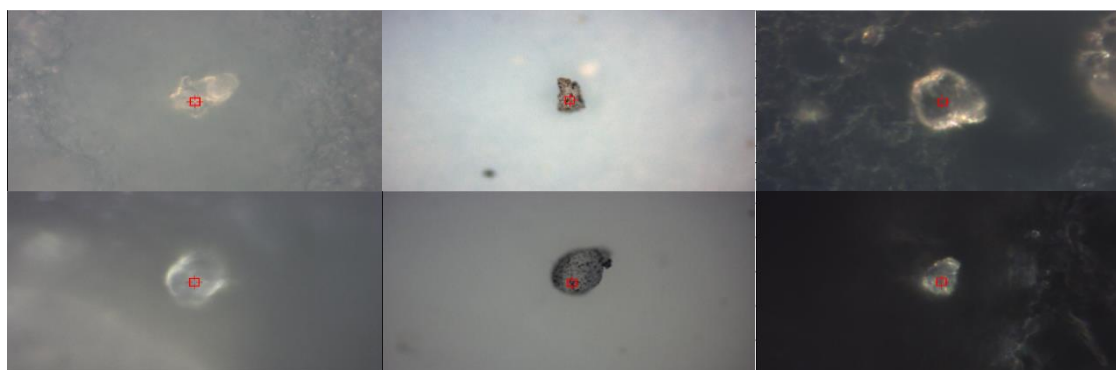
Figure 55. Left to right: particles of sodium nitrate (100x), black powder (10x), and PETN (100x) trapped in the (top to bottom) nitrile and latex materials.
