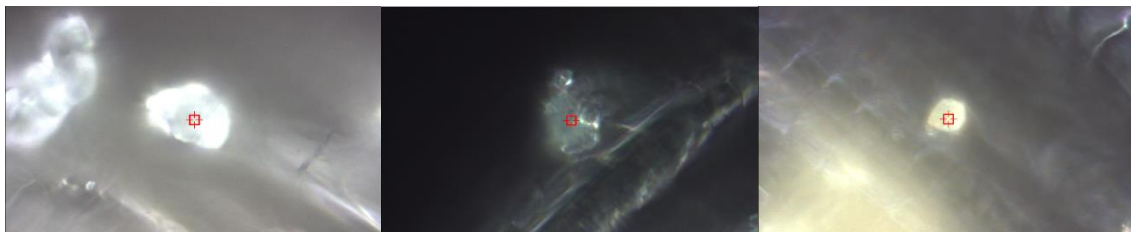
Figure 51. Left to right: particles of ammonium nitrate (100 \times ), chloratite (50 \times ), and TNT (100 \times ) trapped in the wool fibres.
