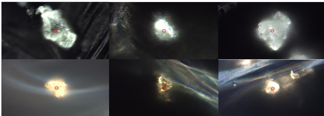
Figure 43. Left to right: particles of potassium nitrate, flash powder, and RDX trapped in the (top to bottom) black and blue polyester fibres (100x).
