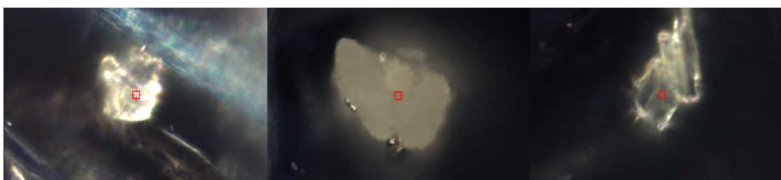
Figure 47. Left to right: particles of sodium chlorate (100x), ammonal (50x), and HMTD (100x) trapped in the blue denim fibres.
