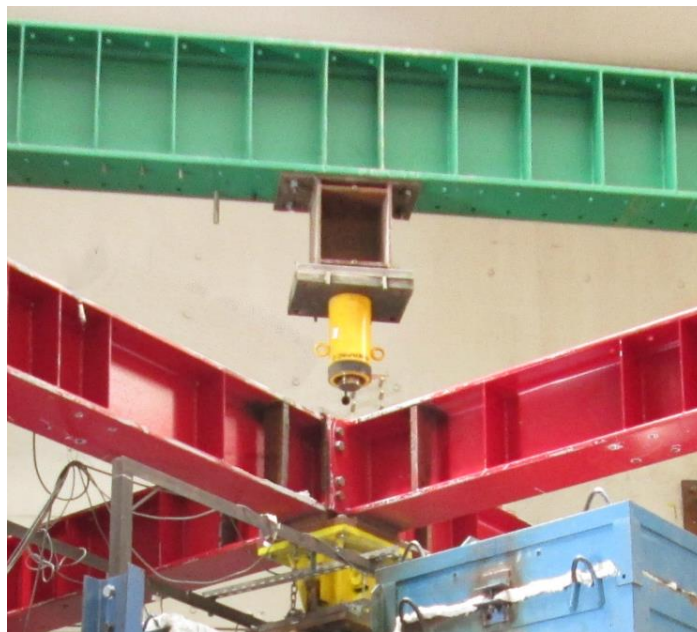
Figure 3.6 - Hydraulic jack just before applying the compression load to the column.
