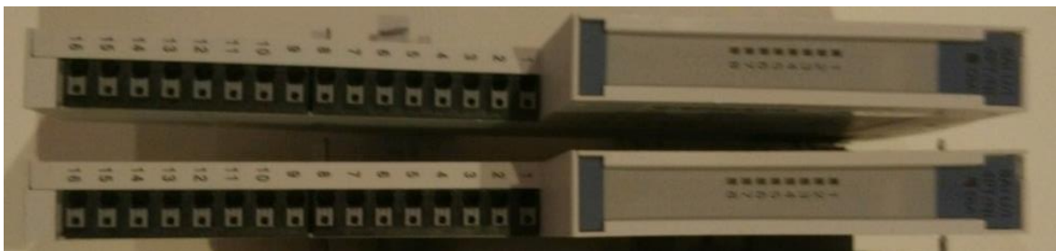
Figura 3.7 – Módulo - “BL20 Economy Module 8 2-wire analog inputs U/I resp. 4 2/3-wire PT/NI inputs BL20-E-8AI-U/I-4PT/NI”
