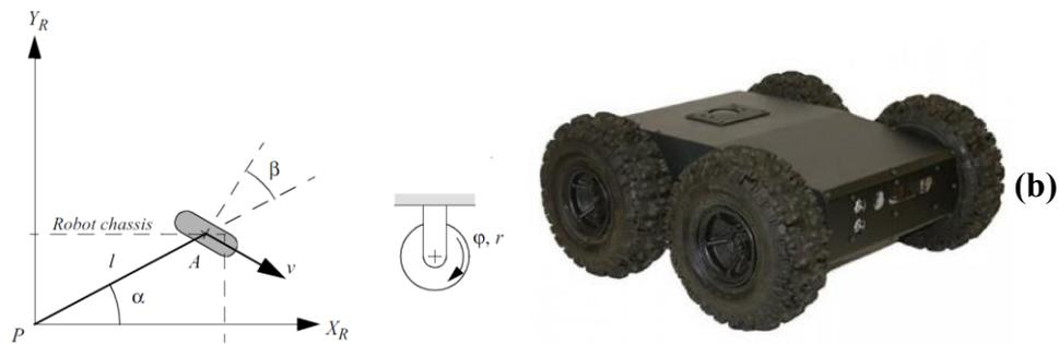
**Figure 2.9.** Kinematics constraints [3] and examples of mobile robots using four wheels as locomotion mechanism: a) steered standard wheel, Adept Mobile Robots Seekur system [21], b) fixed standard wheel, Dr. Robot Jaguar 4x4 Mobile Platform [22].
