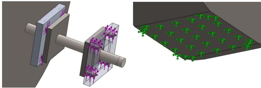
**Figure 3.10.** Model of the robot, forces in purple and restrictions in green.
