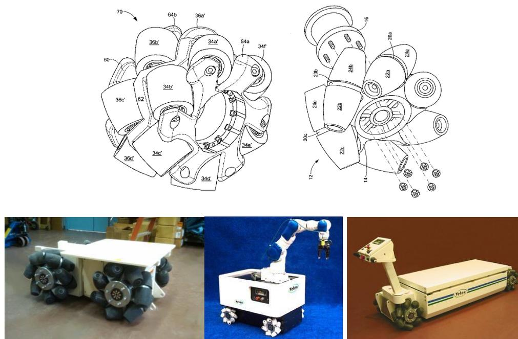
**Figure 2.14.** On the top, we can see two examples of this type of wheels [31] and on the bottom, we have three different robots developed by Vehicle Technologies Inc. [32].
