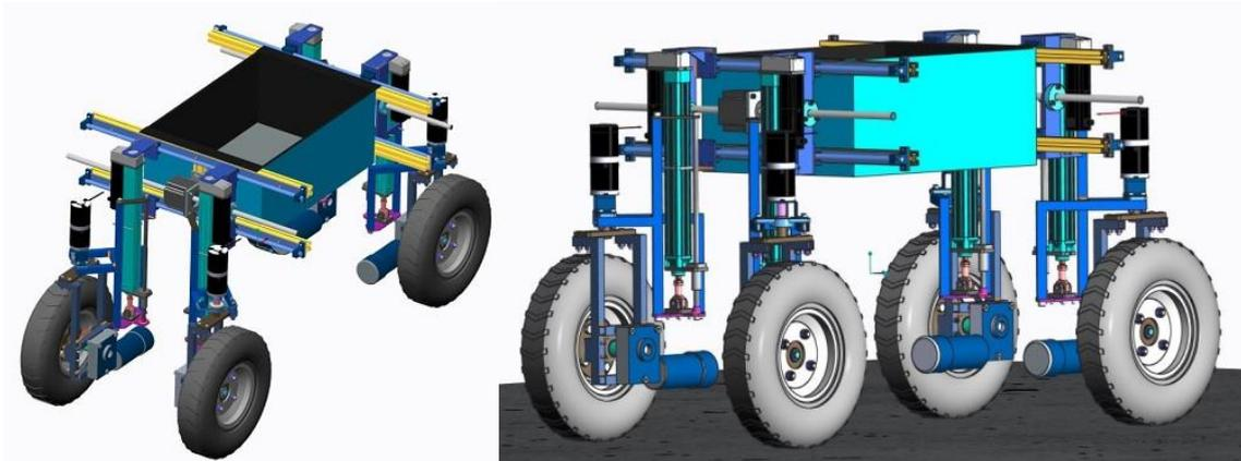
**Figure 2.6.** Modular Multipurpose Omnidirectional Autonomous Mobile Robotic Platform [18].
