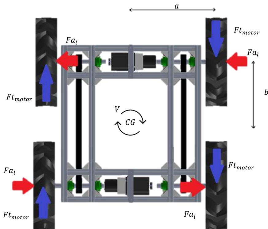
**Figure 3.6.** Top view of the robot; movement around his geometric centre with forces in each wheel.
