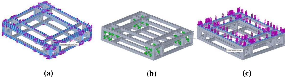
**Figure 3.8.** Simulation made only with the structure that is being developed: a) momentum in purple, b) restrictions in green, c) force representing payload in purple
