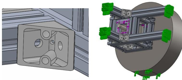
**Figure 3.13.** Automatic-Fastening, one quarter of the structure with restrictions in green and forces in purple.
