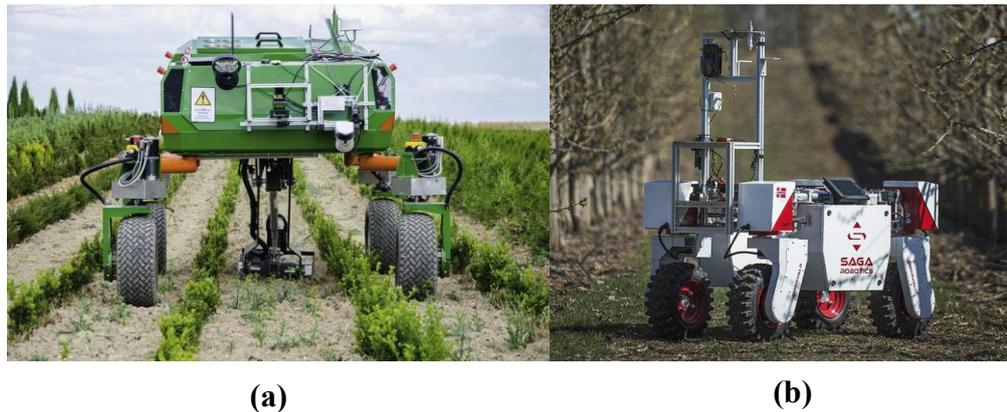
**Figure 1.7.** Mobile robots used in agriculture: a) BoniRob developed by BOSCH Deepfield-Robotics [8], b) Thorvald was desing by SAGA ROBOTICS [9].
