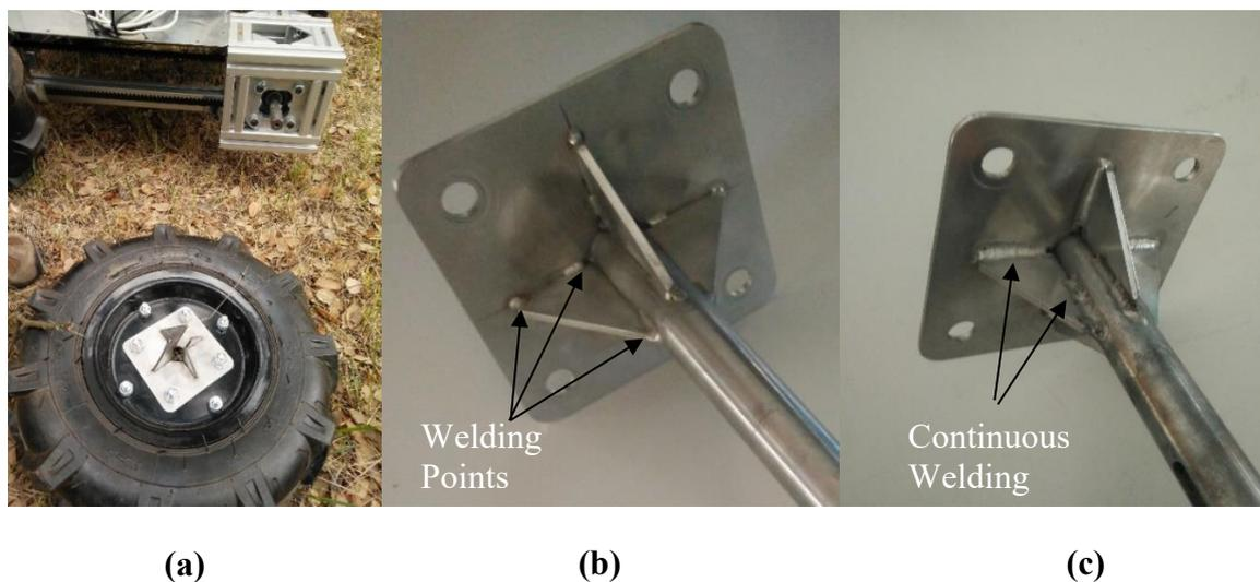
**Figure 4.3.** First problem, testing in rough conditions: a) Broken wheel, b) Shaft before new welding, c) shaft after new welding.
