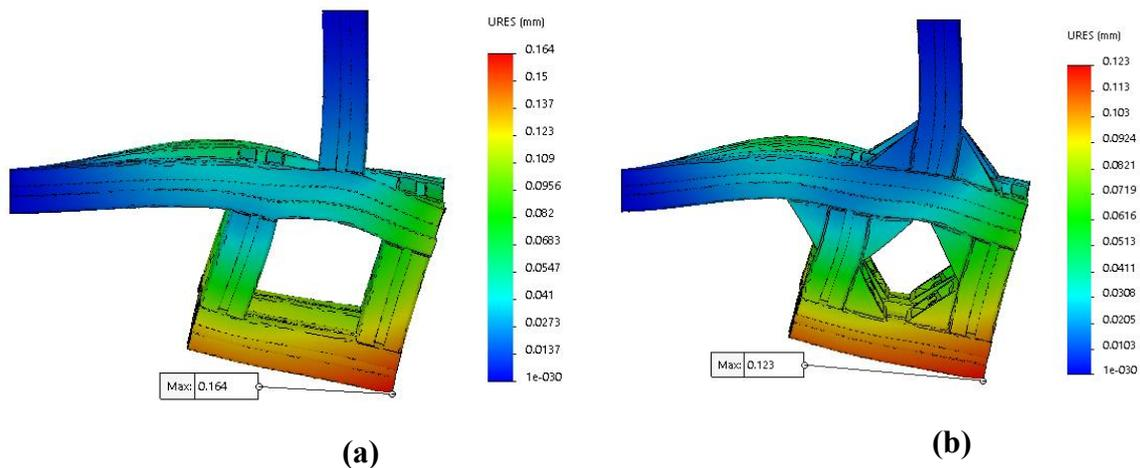
**Figure 3.14.** Deformation results, top view: a) Without fastenings and b) with fastenings.
