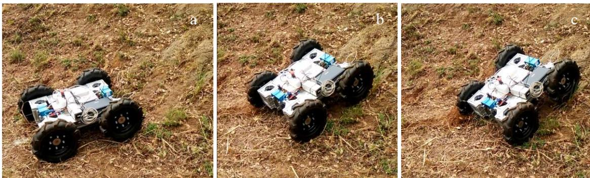
**Figure 4.2.** Video frames of the robot climbing in terrain.
