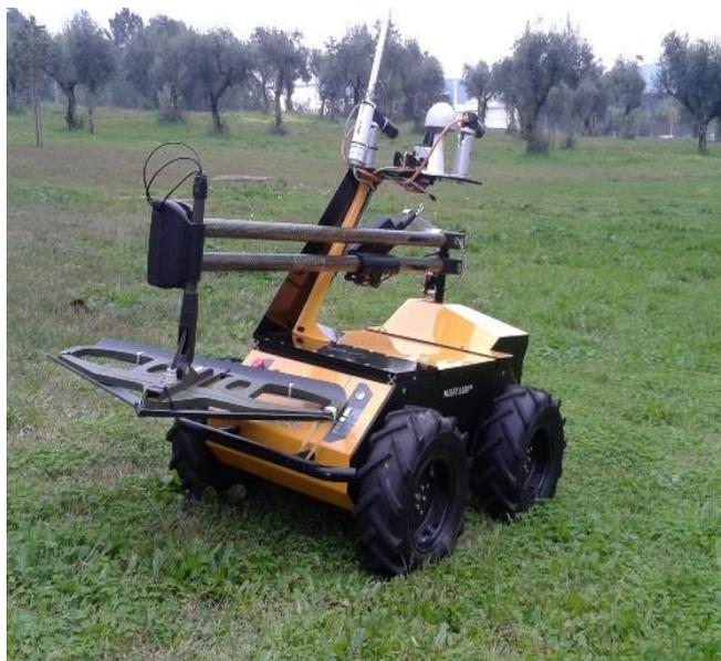
**Figure 1.1.** Husky with mechanisms that make him prepared to detect mines [2].
