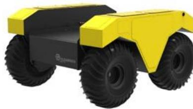
**Figure 2.3.** WARTHOG, amphibious unmanned ground vehicle from Clearpath [15].
