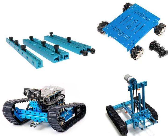
**Figure 2.7.** Robots made with parts from Makeblock [19].
