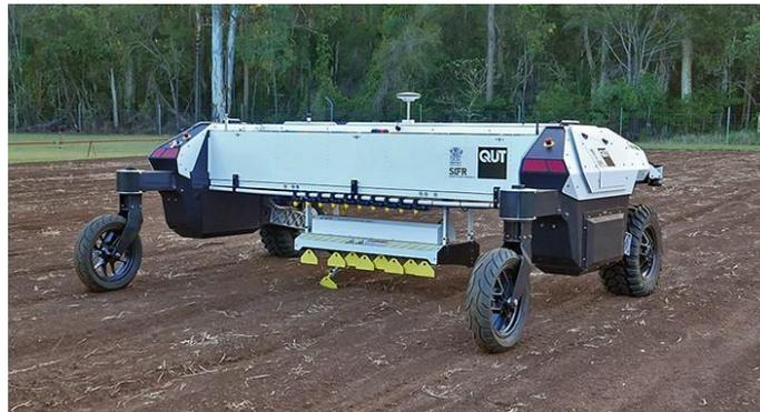
**Figure 2.4.** Small Robotic Farm Vehicle [16].
