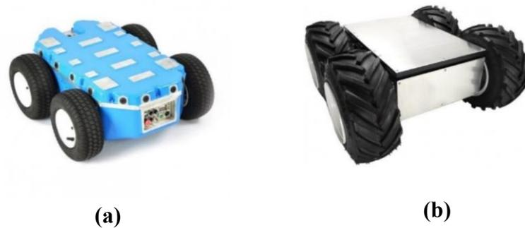
**Figure 2.2.** Sid steer robots with rigid structure: a) Hangfa Navigator C2 Robot Platform [13], b) Inspectorbots Super Mega Bot [14].
