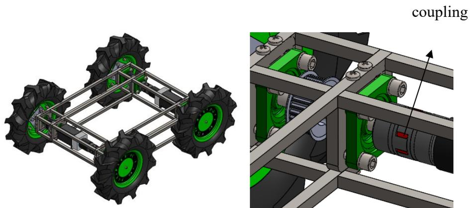
**Figure 3.4.** On the left the first concept for the new mobile robot and on the right the use of a coupling to connect both shafts of the wheel and motor.
