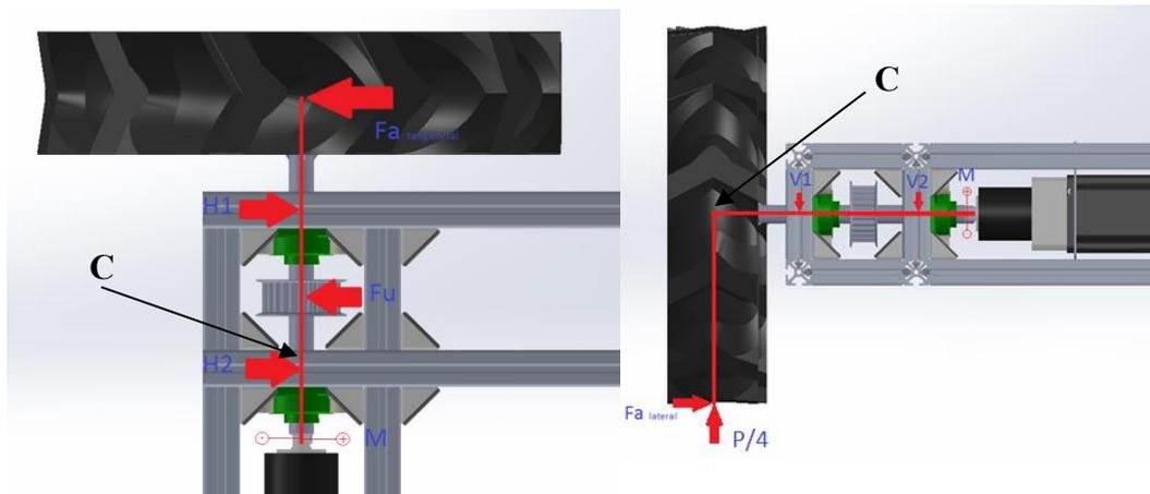
**Figure 3.5.** On the left: top view (horizontal) of one quarter of the robot, and front view (vertical) on the right, both with forces and momentums applied.
