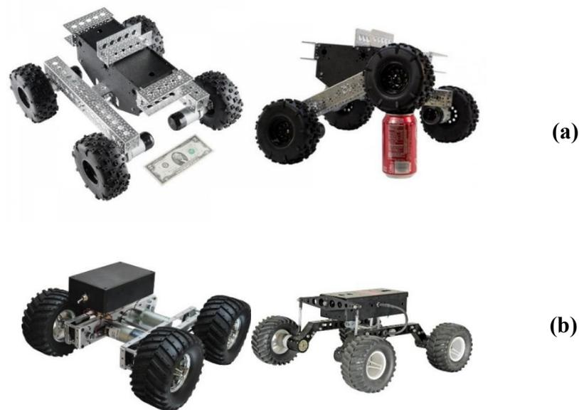
**Figure 2.1.** Skid Steer robots with flexible structure: a) Nomad 4WD Off-Road Chassis Kit [11], b) Gears EdS- Heavy Metal Articulating Chassis (left) and Gears EdS - Surface Mobility Platform (right) [12].
