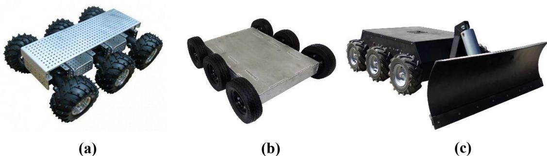
**Figure 2.10.** Mobile robots with six wheels: a) 6WD Wild Mobile Platform [23], b) Super Droid Robots 6WD All Terrain Robot Platform [24], c) Custom RC 6WD Robot with Snow Plow [25].
