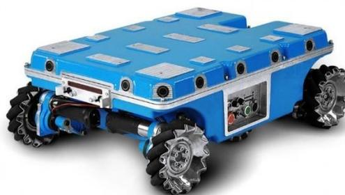
**Figure 2.16.** Hangfa Navigator Q2 Robot Platform, with four 45 degrees QMA-15 omni wheels [36].
