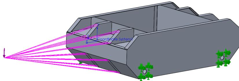
**Figure 3.2.** Simulation made to secure the safety of the structure with a remote load.
