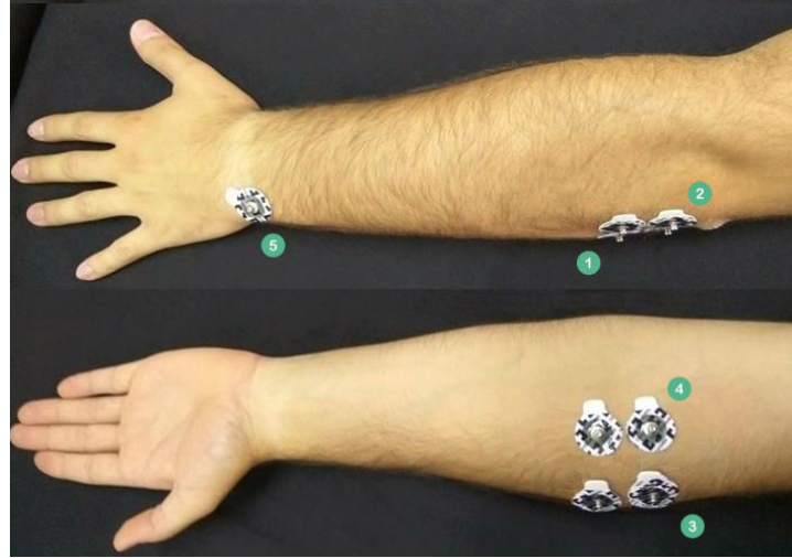
Figure 3.8: Electrode placement during gesture classification, where the 5th sensor corresponds to the reference electrode.
