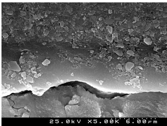
Figure 21: SEM image of adhesive interface of group 3 (Al 2 O 3 + SBU) (5000x)
