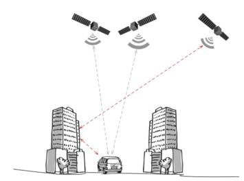
Figure 8: GNSS Multipath Errors
