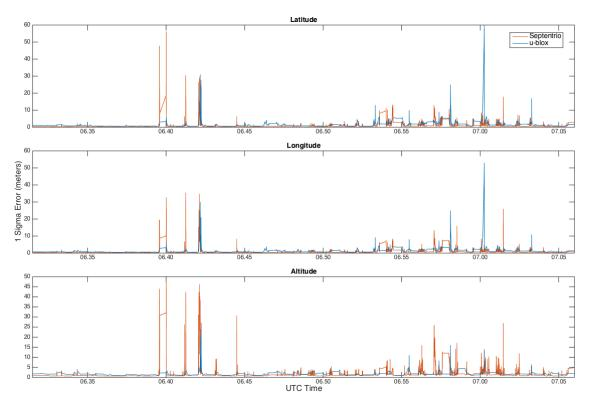
Figure 24: Latitude, Longitude and Altitude - 1 Sigma Errors
