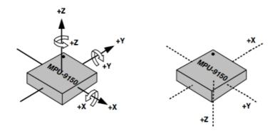
Figure 15: MPU-9150 Accelerometer/Gyroscope and Magnetometer Axes Orientation
