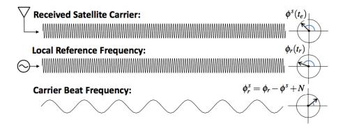
Figure 7: GPS Carrier Phase [Takasu, 2015]
