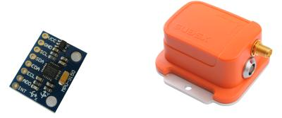
Figure 9: InvenSense MPU-9150 and Xsens MTi-G
