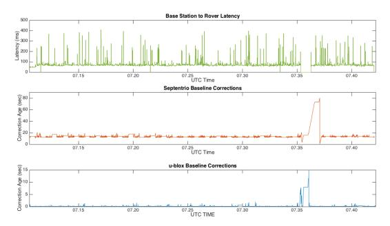
Figure 38: Latency between the Base Stations and the Rover, RTK Correction Age
