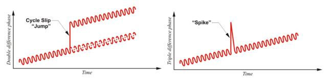
Figure 51: GNSS Cycle Slip [Sickle, 2014]
