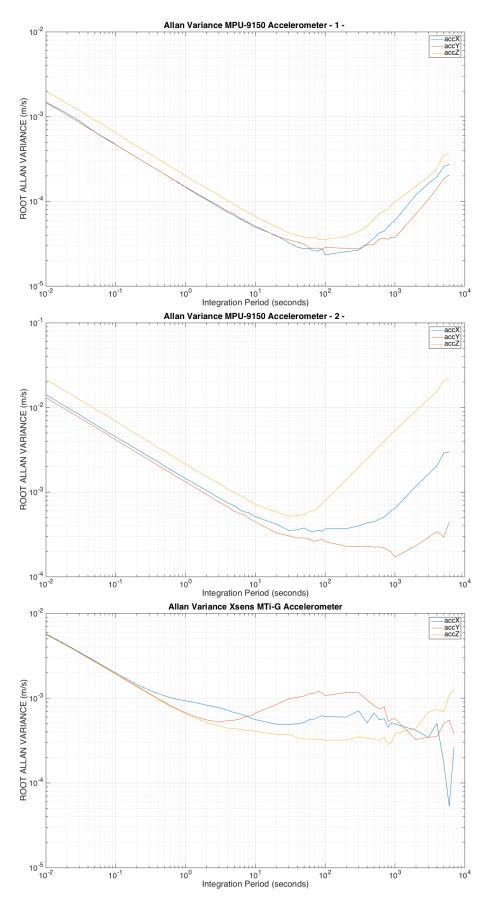
Figure 48: Allan Variance for Raw Accelerometer Data
