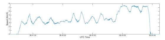
Figure 42: RTK Low Speed Test - Velocity reported by the Septentrio AsteRx4 Receiver
