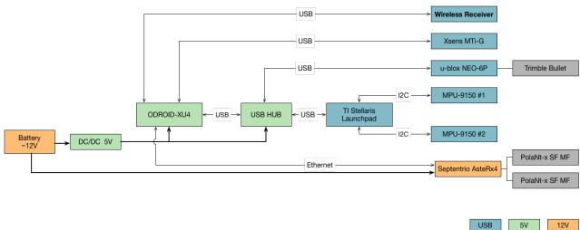
Figure 45: Rover Connections Diagram
