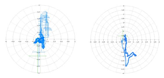
Figure 19: Septentrio (left) and u-blox (right) Base Stations Position Random Walk
