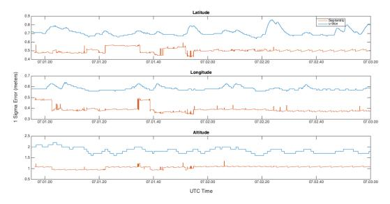
Figure 31: Low Speed Test - 1 Sigma Error
