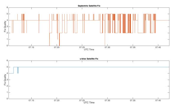
Figure 35: RTK GNSS Receivers Fix Quality
