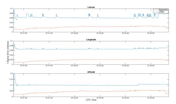
Figure 44: RTK Low Speed Test - 1 Sigma Error
