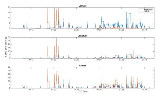
Figure 36: RTK Latitude, Longitude and Altitude - 1 Sigma Errors
