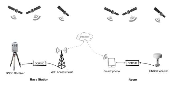
Figure 16: RTK-GNSS Connection Diagram
