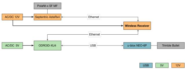
Figure 46: Base Station Connections Diagram
