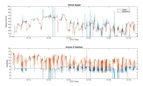
Figure 32: RTK Vehicle Speed and Number of Satellites
