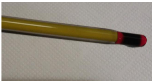
Figure 11 Aggregates of MWCNTs after dispersion of 0.01% (w/w) of MWCNTs with polyDADMAC MMW at a concentration of 0.03% (w/w).
