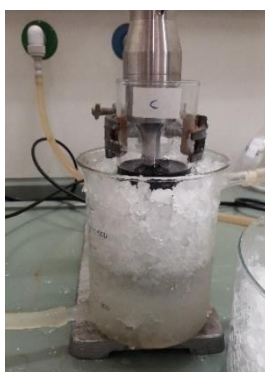
Figure 10 Ice bath with water flux prepared during MWCNTs dispersions, using an ultrasound equipment.
